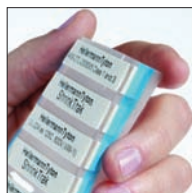
Step 2 Bend liner at side slit
