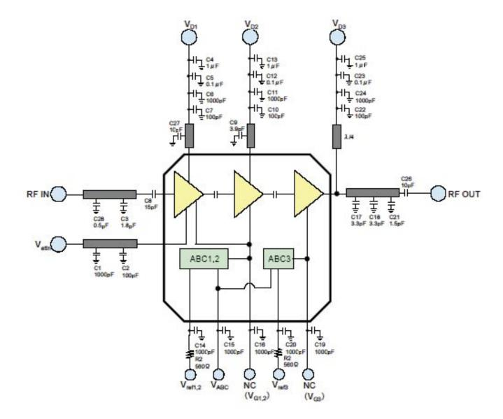
NC (VG1,2 VG3) These pins must be connected to ground via a 1000pF capacitor for stability.
