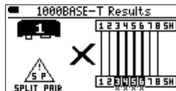
Typical split pair wiring fault
