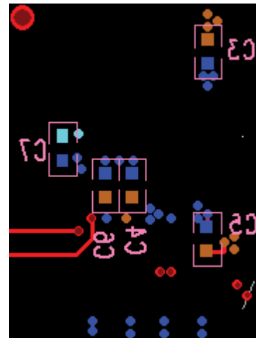
Figure 53. Bottom Layer Decoupling
