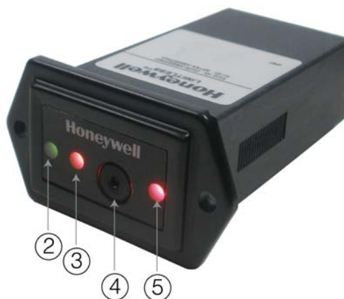
Figure 9. Limitless™ WPMM LED display
