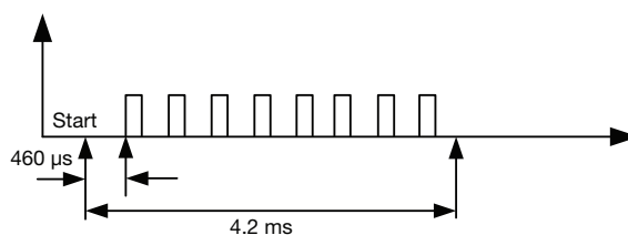
Fig. 18 - Ambient Light Measurement with Averaging = 8; using Continuous Conversion Mode
