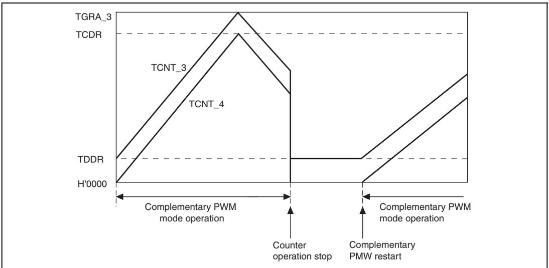
**Figure 9.119 Counter Value during Complementary PWM Mode Stop**
