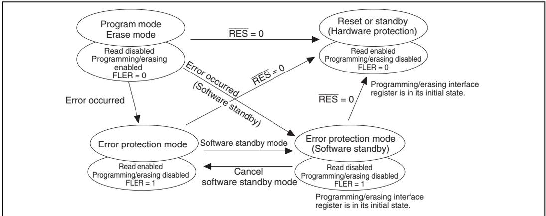
**Figure 17.13 Transitions to and from Error Protection State**
