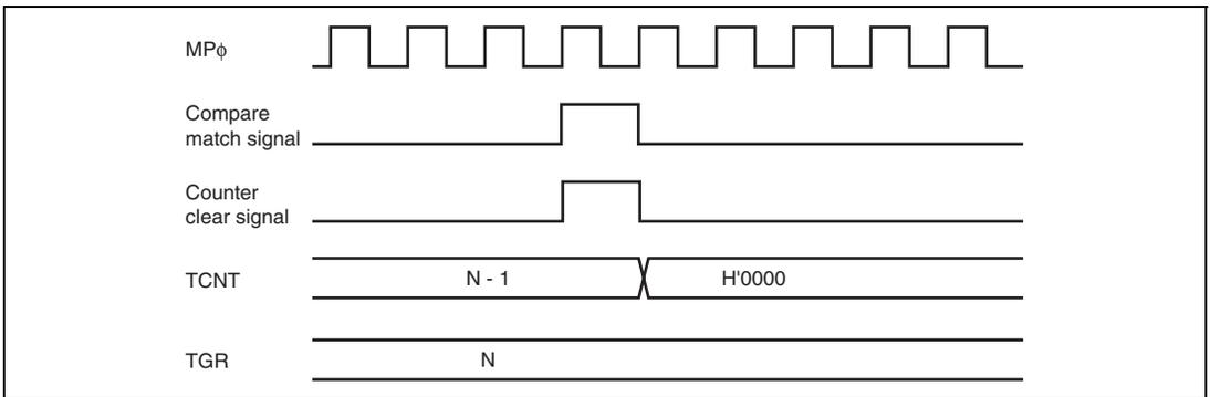
**Figure 9.91 Counter Clear Timing (Compare Match) (Channel 5)**
