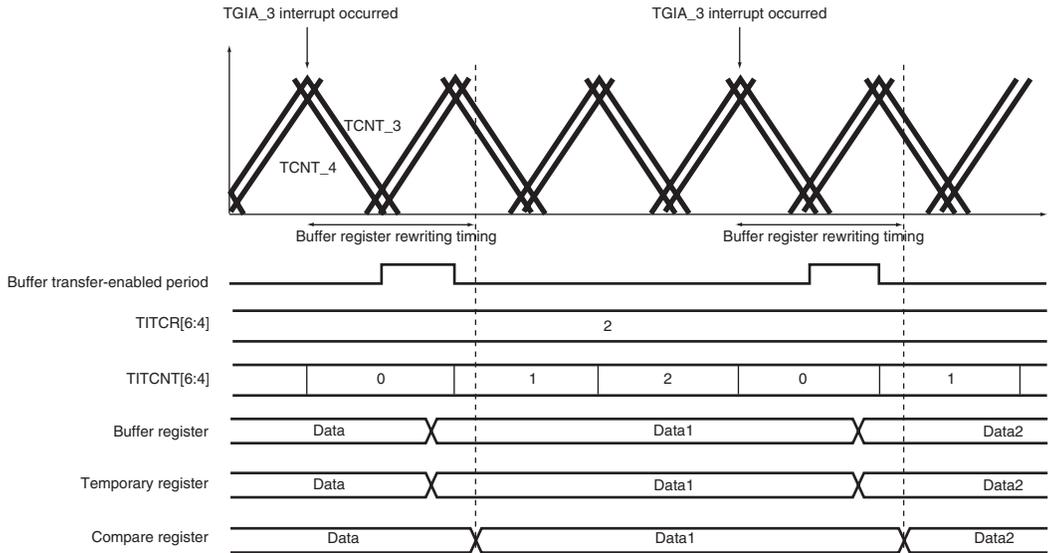
(2) When rewriting a buffer register after a carrier cycle passed from occurring TGIA\_3 interrupt.
