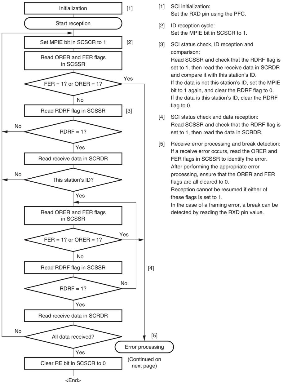
Figure 12.18 Sample Multiprocessor Serial Reception Flowchart (1)
