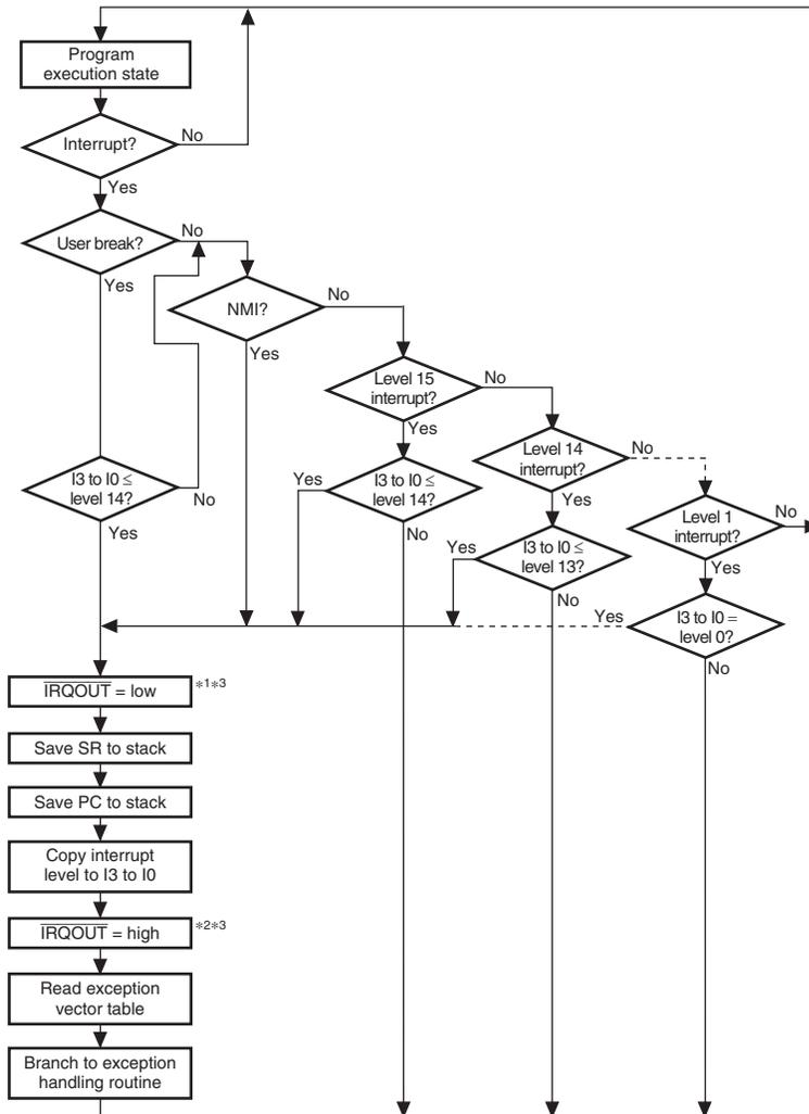
Notes: I3 to I0 are interrupt mask bits in the status register (SR) of the CPU
