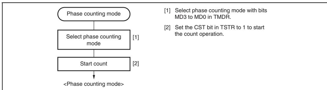
**Figure 9.29 Example of Phase Counting Mode Setting Procedure**
