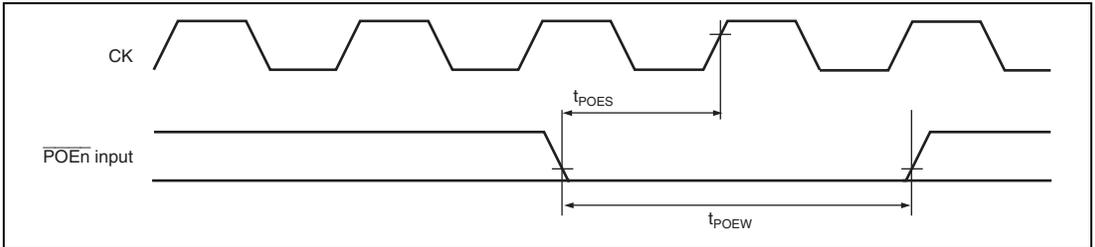
**Figure 21.14 POE Input Timing**
