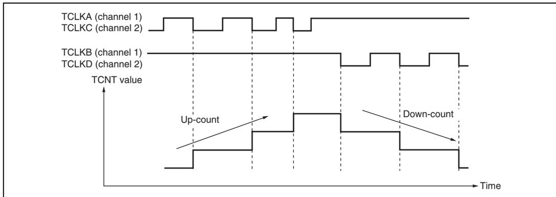
**Figure 9.32 Example of Phase Counting Mode 3 Operation**
