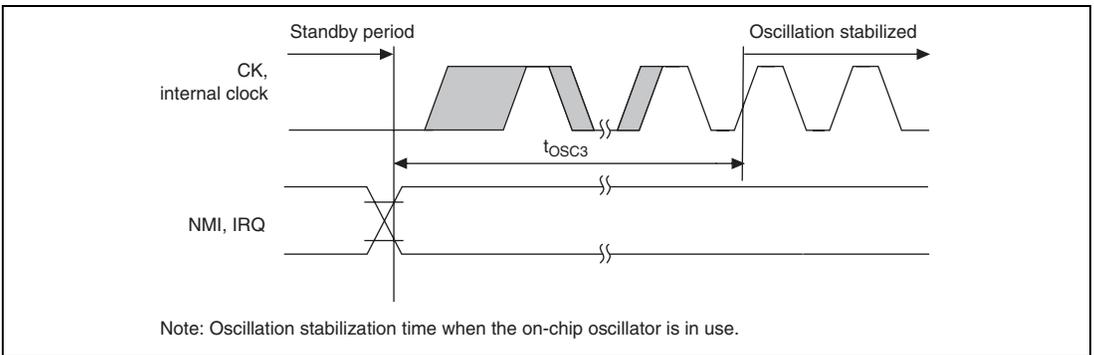
**Figure 21.4 Oscillation Stabilization Time on Return from Standby (Return by NMI or IRQ)**
