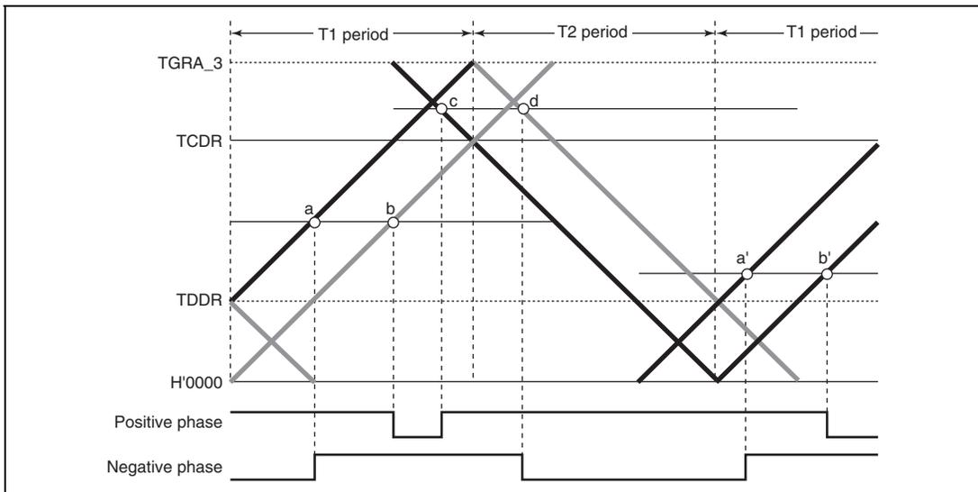
**Figure 9.46 Example of Complementary PWM Mode Waveform Output (1)**
