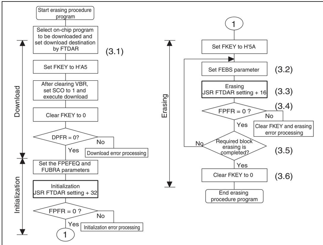
**Figure 17.12 Erasing Procedure**
