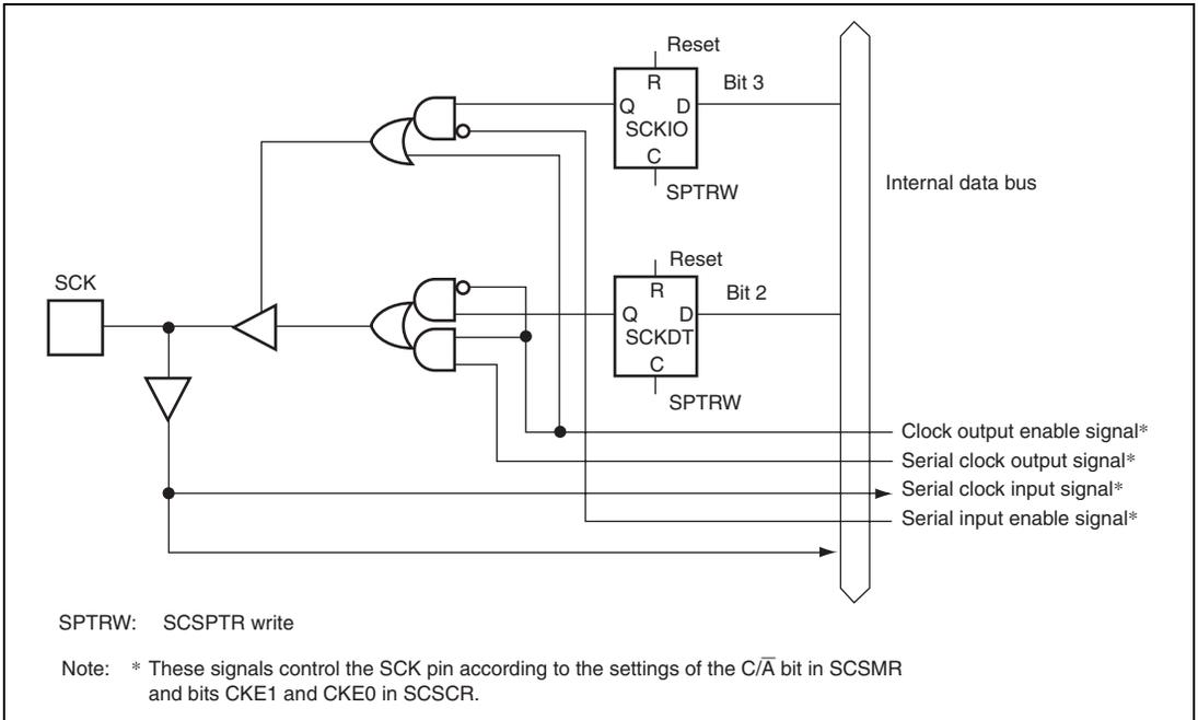
**Figure 12.19** SPB1IO bit, SPB1DT bit, and SCK Pin
