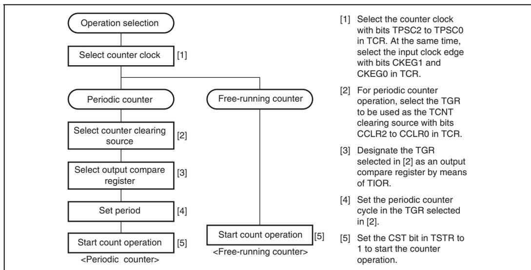
**Figure 9.4 Example of Counter Operation Setting Procedure**
