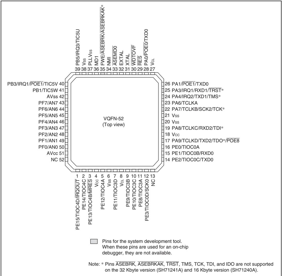
**Figure 1.3 (2) Pin Assignments of SH7124**
