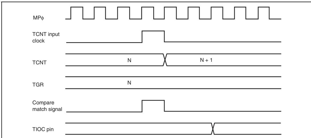
**Figure 9.88 Output Compare Output Timing**
