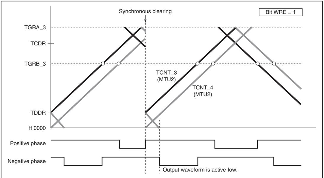
**Figure 9.59 Example of Synchronous Clearing in Interval Tb at Crest
