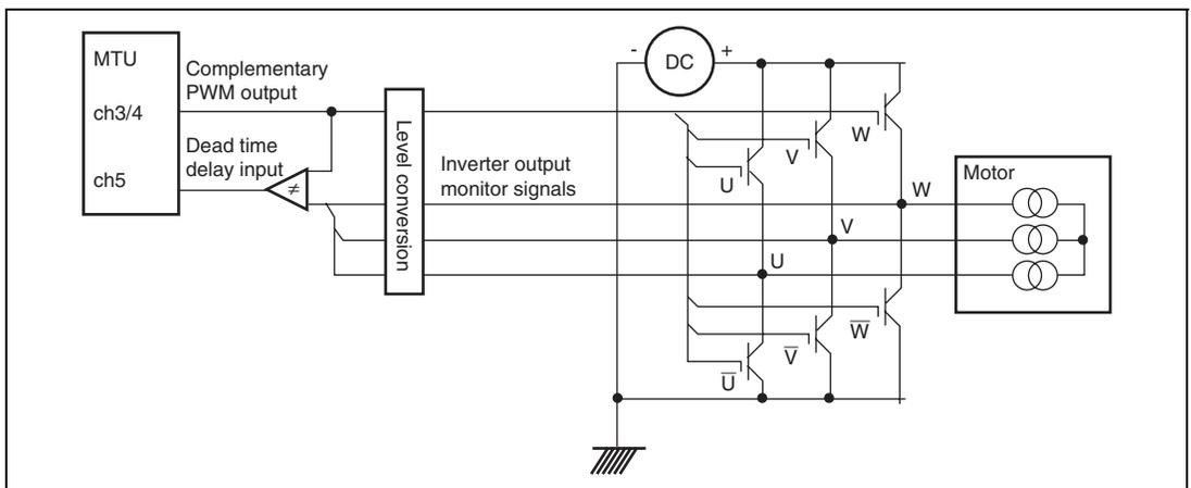
**Figure 9.81 Example of Motor Control Circuit Configuration**
