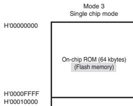
Figure 3.3 Address Map in SH71251A and SH71241A (32 Kbytes Flash Memory Version) 53 Figure amended
