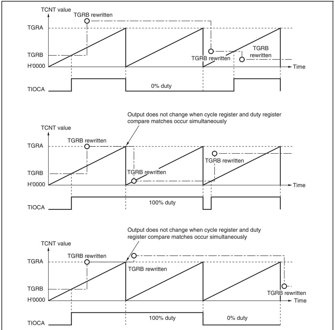
**Figure 9.28 Example of PWM Mode Operation (3)**
