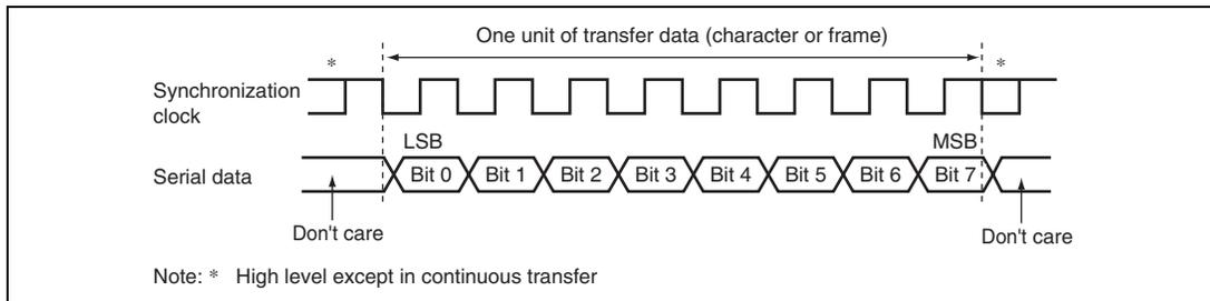
**Figure 12.8 Data Format in Clock Synchronous Communication**
