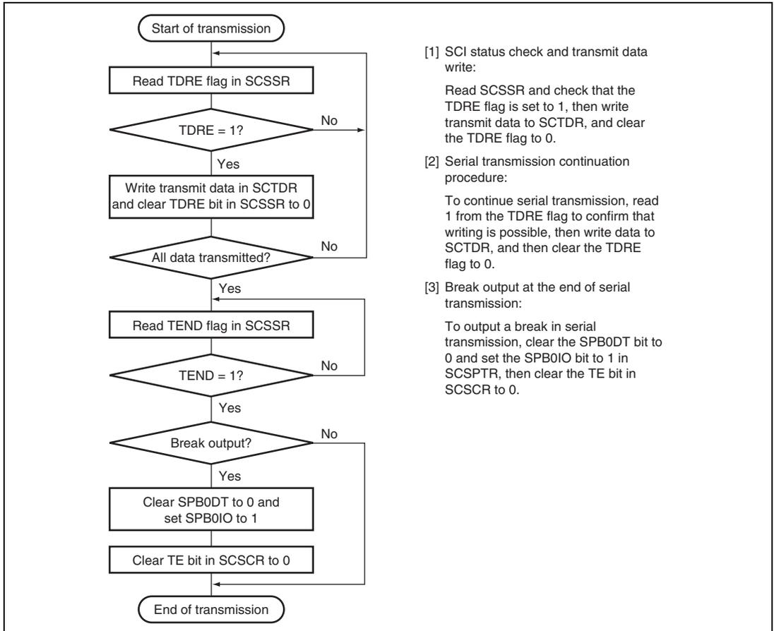
**Figure 12.4 Sample Flowchart for Transmitting Serial Data**
