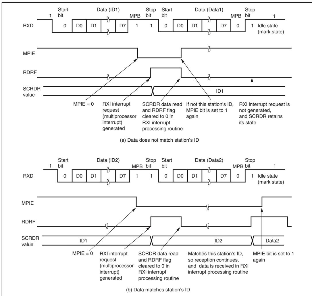
**Figure 12.17 Example of SCI Operation in Reception
