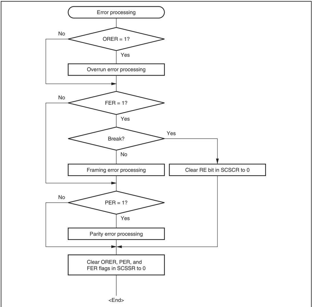
**Figure 12.6 Sample Flowchart for Receiving Serial Data (cont)**
