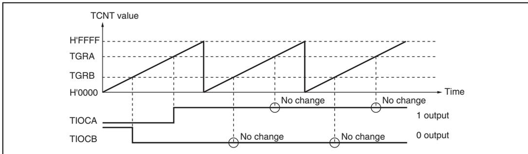
**Figure 9.8 Example of 0 Output/1 Output Operation**
