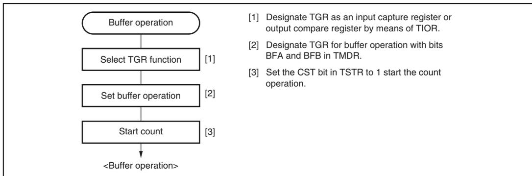
**Figure 9.16 Example of Buffer Operation Setting Procedure**
