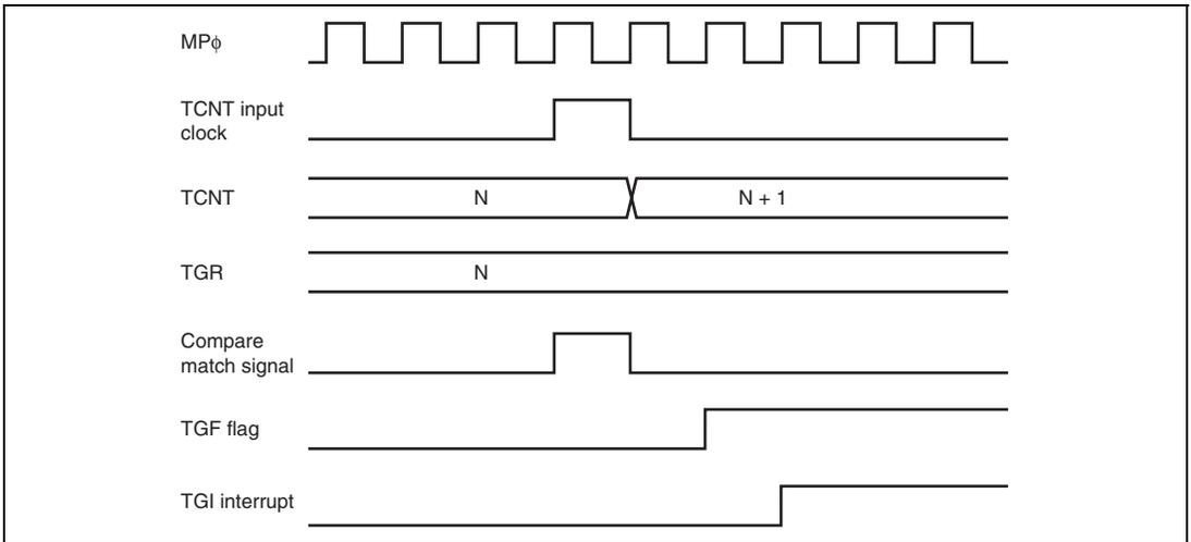
**Figure 9.99 TGI Interrupt Timing (Compare Match) (Channels 0 to 4)**
