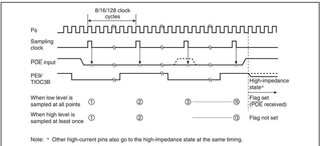
**Figure 10.3 Low-Level Detection Operation**
