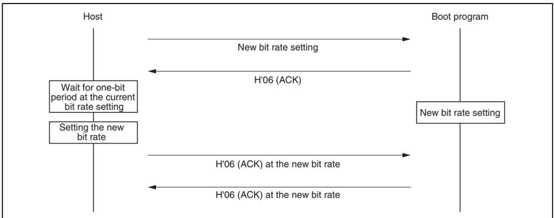
**Figure 17.18 Sequence of New Bit Rate Selection**
