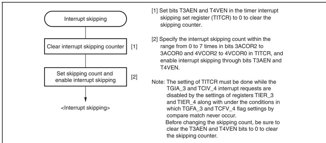
**Figure 9.67 Example of Interrupt Skipping Operation Setting Procedure**
