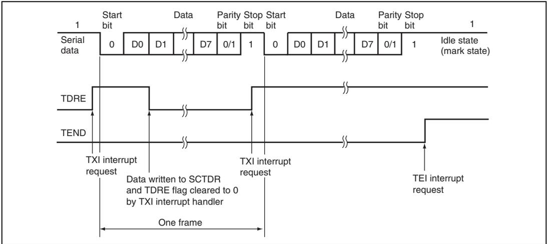
**Figure 12.5 Example of Transmission in Asynchronous Mode
