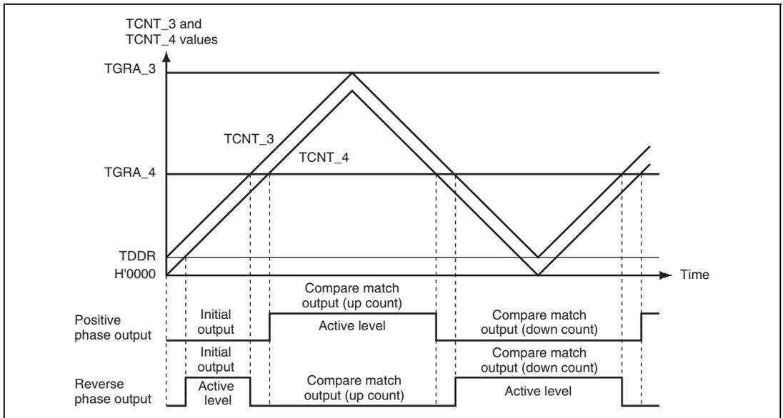
**Figure 9.2 Complementary PWM Mode Output Level Example**
