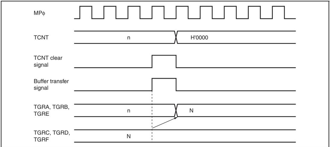
**Figure 9.95 Buffer Transfer Timing (when TCNT Cleared)**
