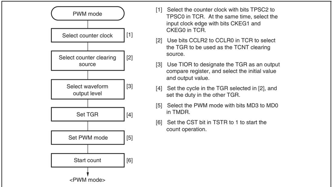
**Figure 9.25 Example of PWM Mode Setting Procedure**
