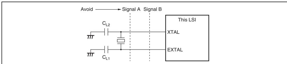
**Figure 4.5 Cautions for Oscillator Circuit Board Design**
