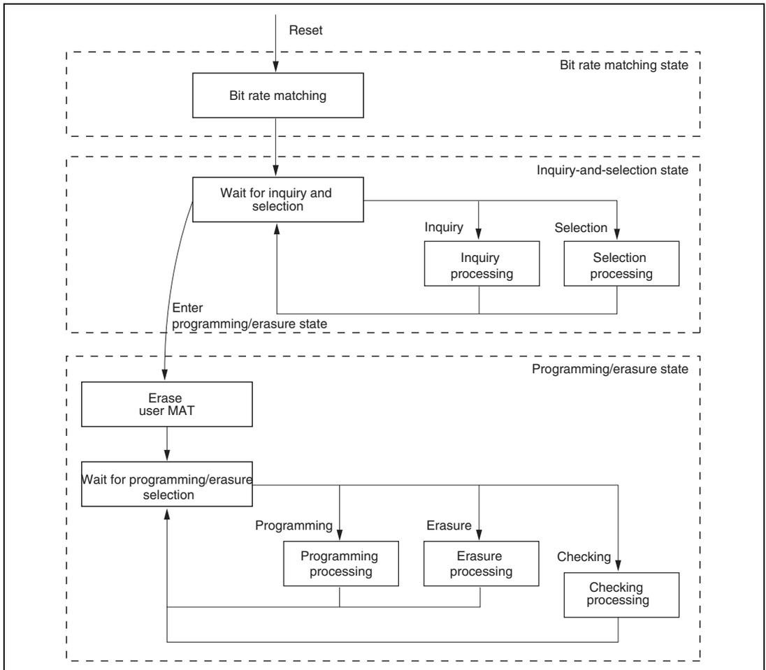
**Figure 17.15 Flow of Processing by the Boot Program**
