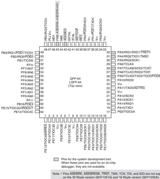
Figure 1.2 (2) Pin Assignments of SH7125
