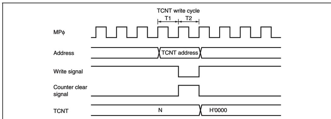
**Figure 9.108 Contention between TCNT Write and Clear Operations**
