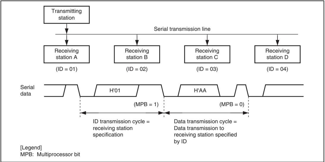
**Figure 12.15 Example of Communication Using Multiprocessor Format
