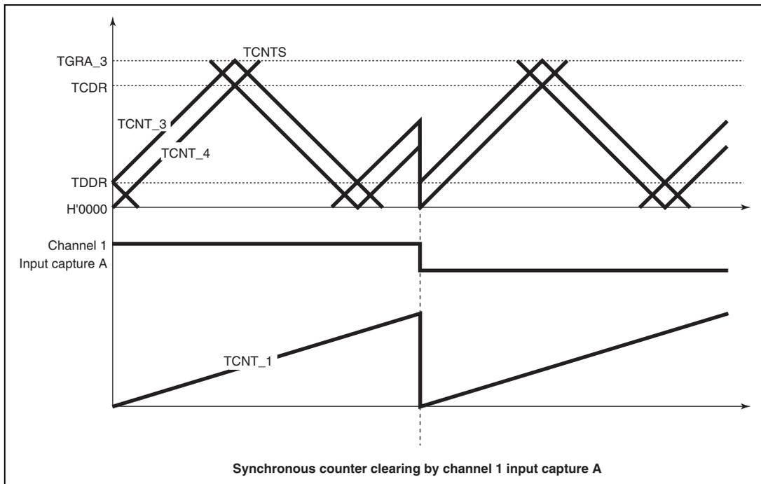
**Figure 9.55 Counter Clearing Synchronized with Another Channel**
