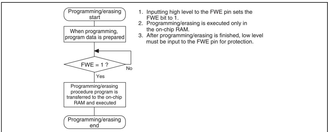
**Figure 17.9 Programming/Erasing Overview Flow**
