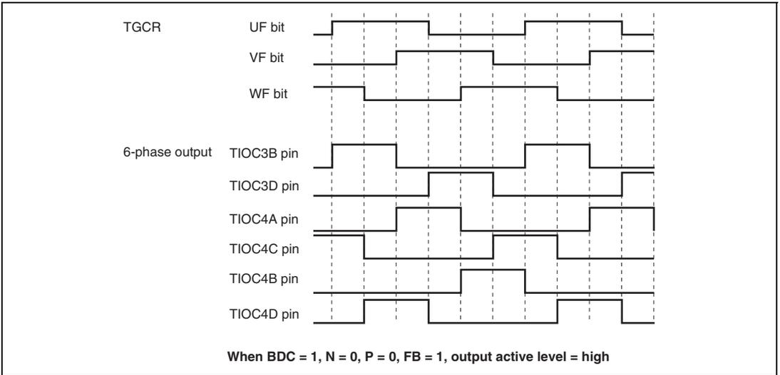
**Figure 9.65 Example of Output Phase Switching by Means of UF, VF, WF Bit Settings (1)**
