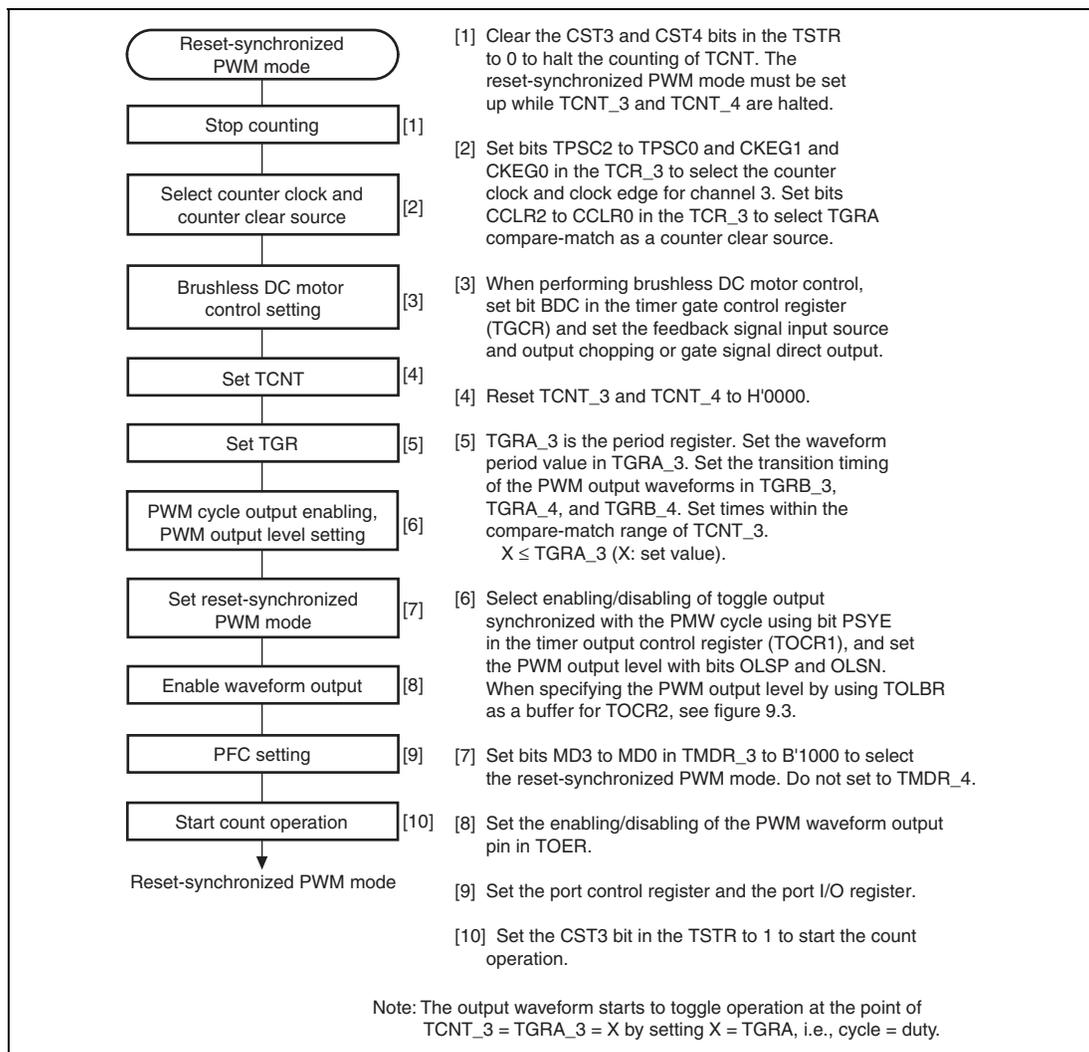
**Figure 9.35 Procedure for Selecting Reset-Synchronized PWM Mode**
