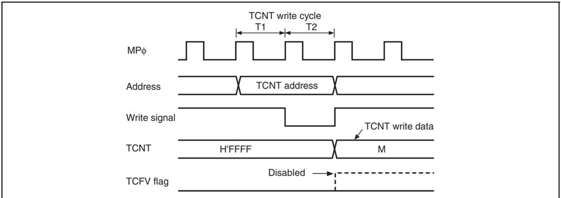
**Figure 9.123 Contention between TCNT Write and Overflow**
