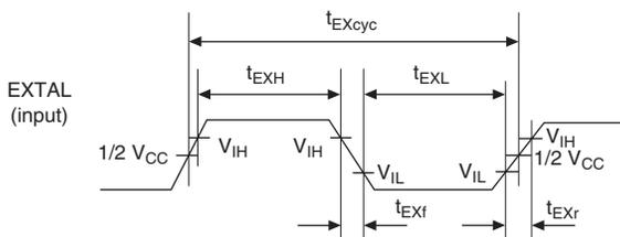
**Figure 21.1 Timing of EXTAL Input Clock Signal**
