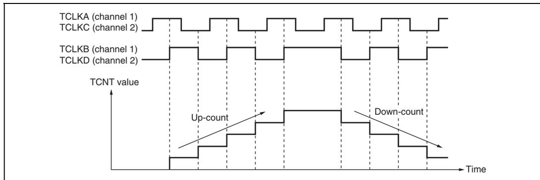
**Figure 9.33 Example of Phase Counting Mode 4 Operation**
