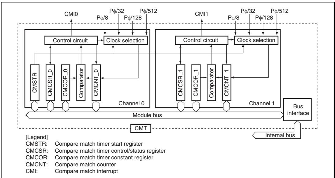
Figure 14.1 Block Diagram of CMT
