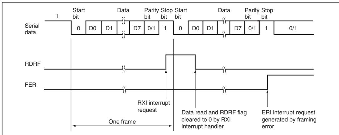
**Figure 12.7 Example of SCI Receive Operation
