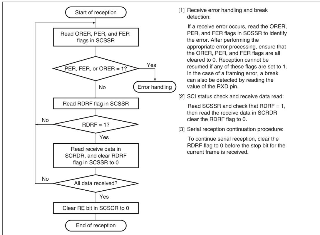
**Figure 12.6 Sample Flowchart for Receiving Serial Data**
