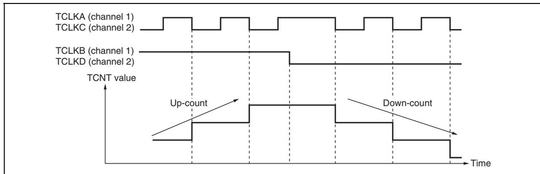
**Figure 9.31 Example of Phase Counting Mode 2 Operation**
