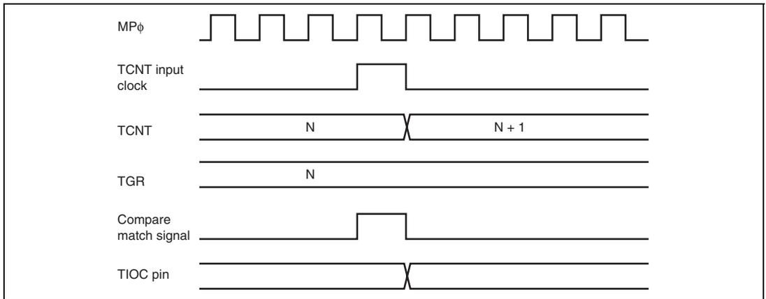
**Figure 9.87 Output Compare Output Timing (Normal Mode/PWM Mode)**
