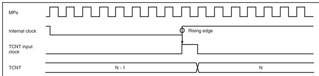
**Figure 9.84 Count Timing in Internal Clock Operation (Channel 5)**
