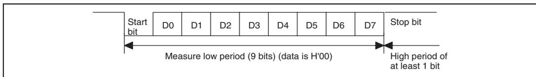
**Figure 17.7 Automatic Adjustment Operation of SCI Bit Rate**
