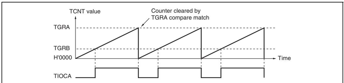
**Figure 9.26 Example of PWM Mode Operation (1)**
