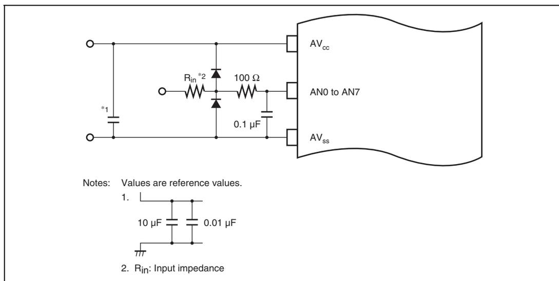
Figure 13.8 Example of Analog Input Protection Circuit
