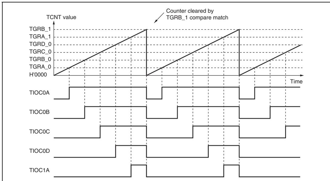
**Figure 9.27 Example of PWM Mode Operation (2)**
