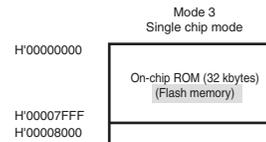
Figure 3.4 Address Map in SH71250A and SH71240A (16 Kbytes Flash Memory Version) 54 Figure added
