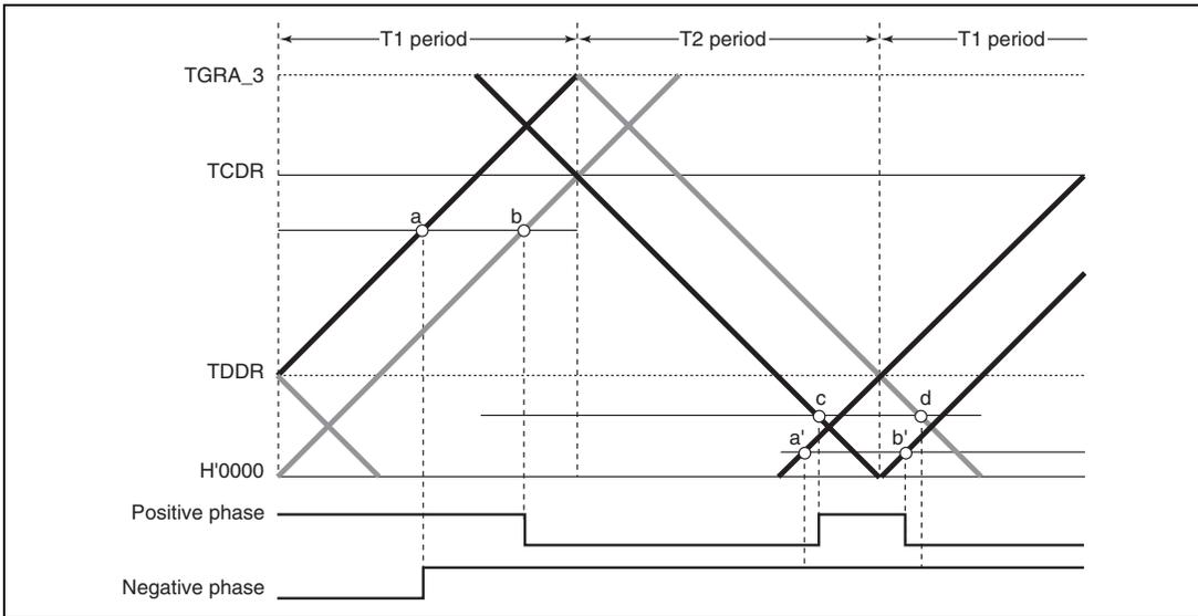
**Figure 9.48 Example of Complementary PWM Mode Waveform Output (3)**
