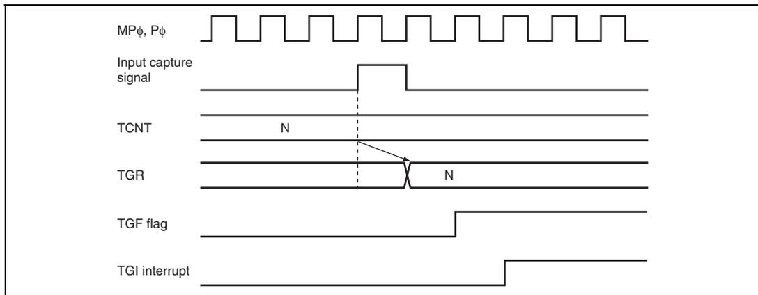
**Figure 9.101 TGI Interrupt Timing (Input Capture) (Channels 0 to 4)**
