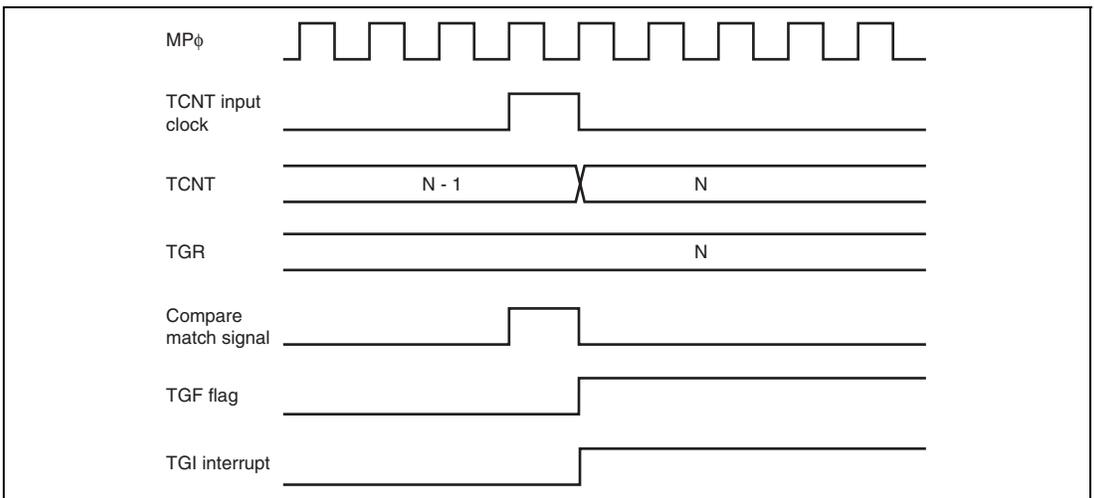
**Figure 9.100 TGI Interrupt Timing (Compare Match) (Channel 5)**
