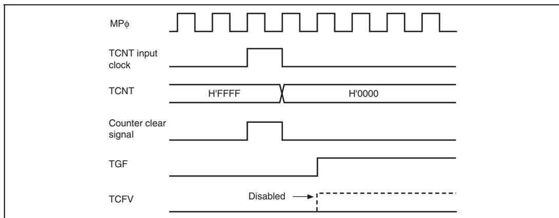
**Figure 9.122 Contention between Overflow and Counter Clearing**
