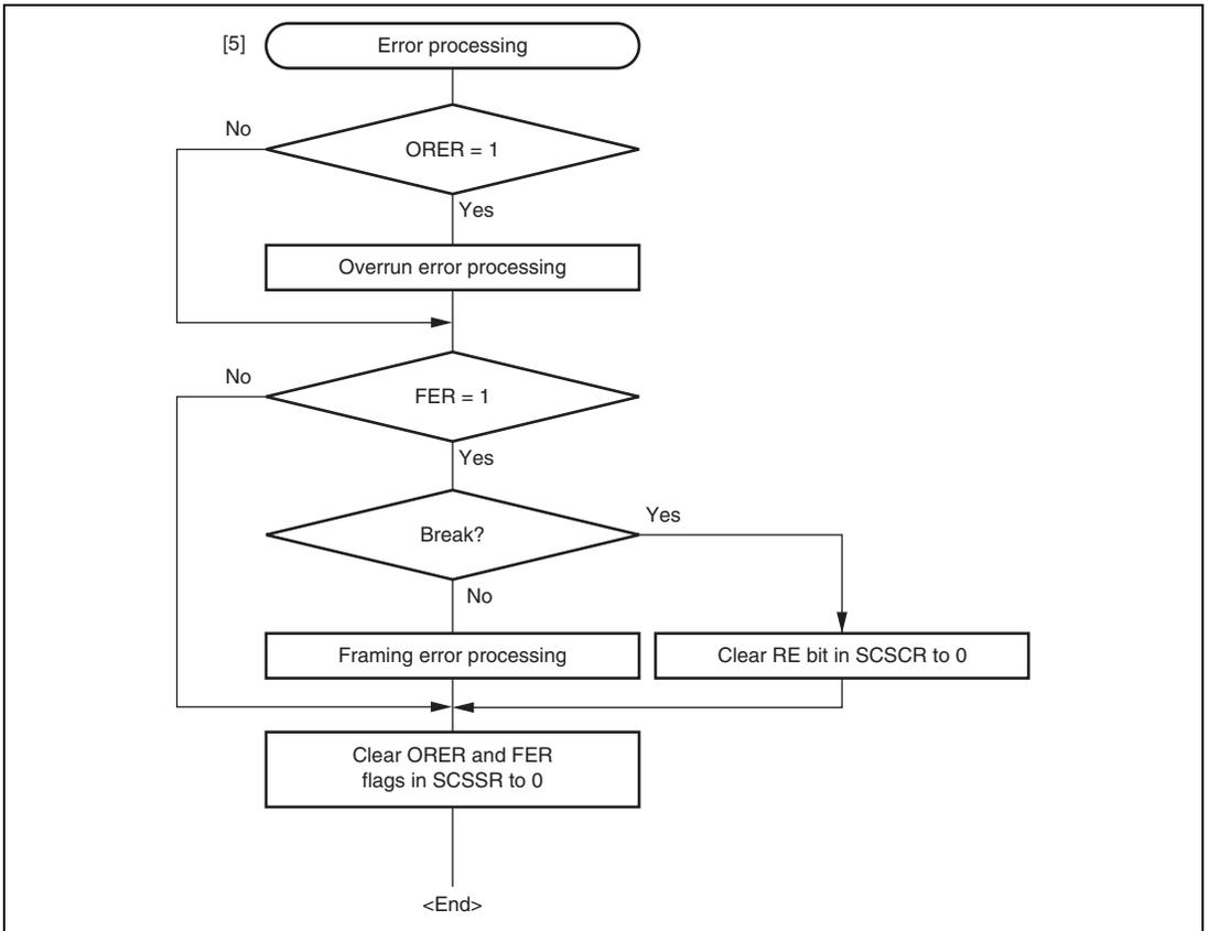
**Figure 12.18 Sample Multiprocessor Serial Reception Flowchart (2)**
