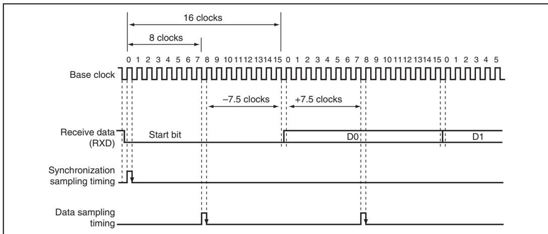
**Figure 12.21 Receive Data Sampling Timing in Asynchronous Mode**
