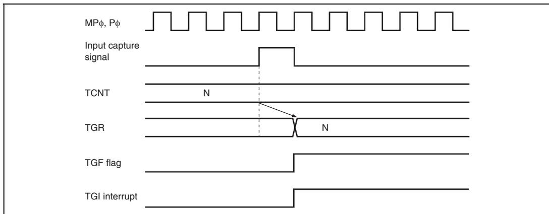
**Figure 9.102 TGI Interrupt Timing (Input Capture) (Channel 5)**
