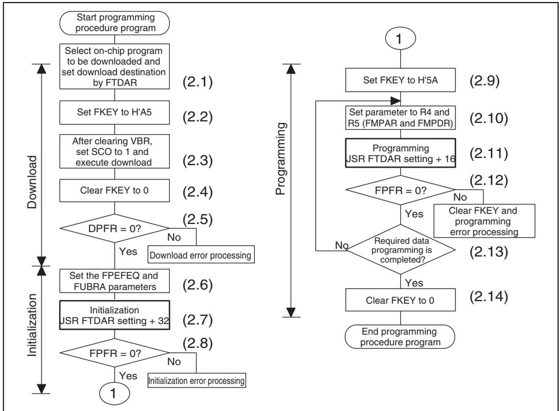
**Figure 17.11 Programming Procedure**
