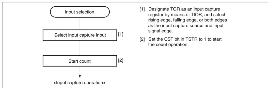
**Figure 9.10 Example of Input Capture Operation Setting Procedure**
