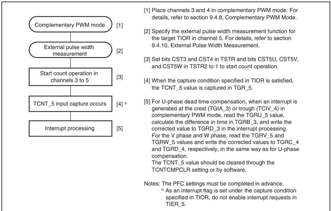
**Figure 9.80 Example of Dead Time Compensation Setting Procedure**
