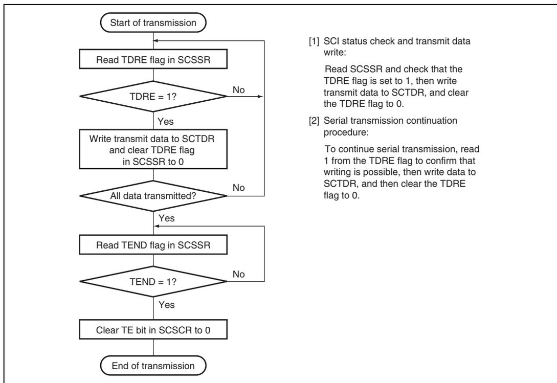
**Figure 12.10 Sample Flowchart for Transmitting Serial Data**
