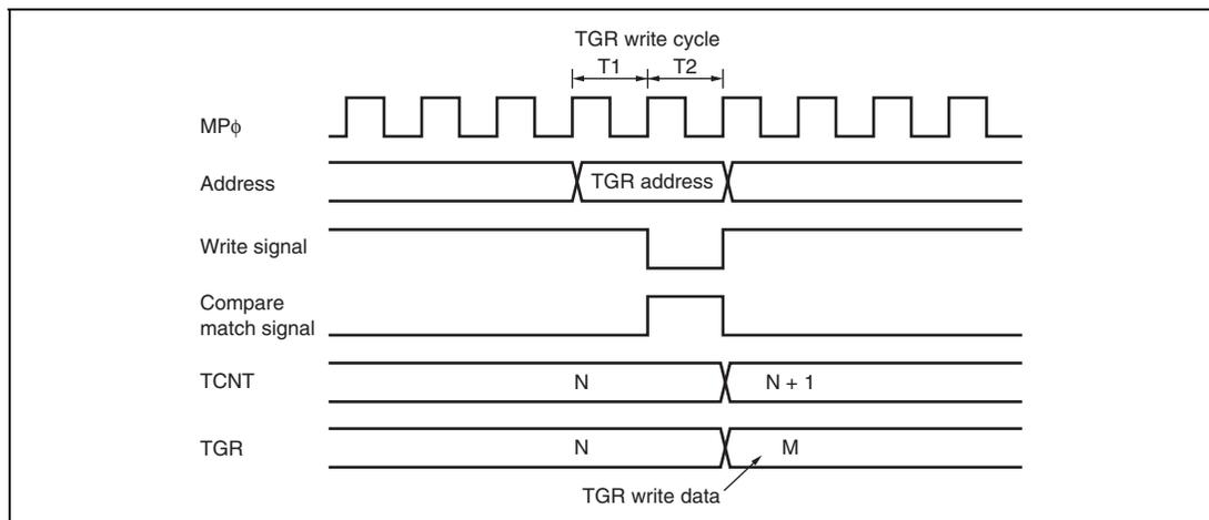
**Figure 9.110 Contention between TGR Write and Compare Match**
