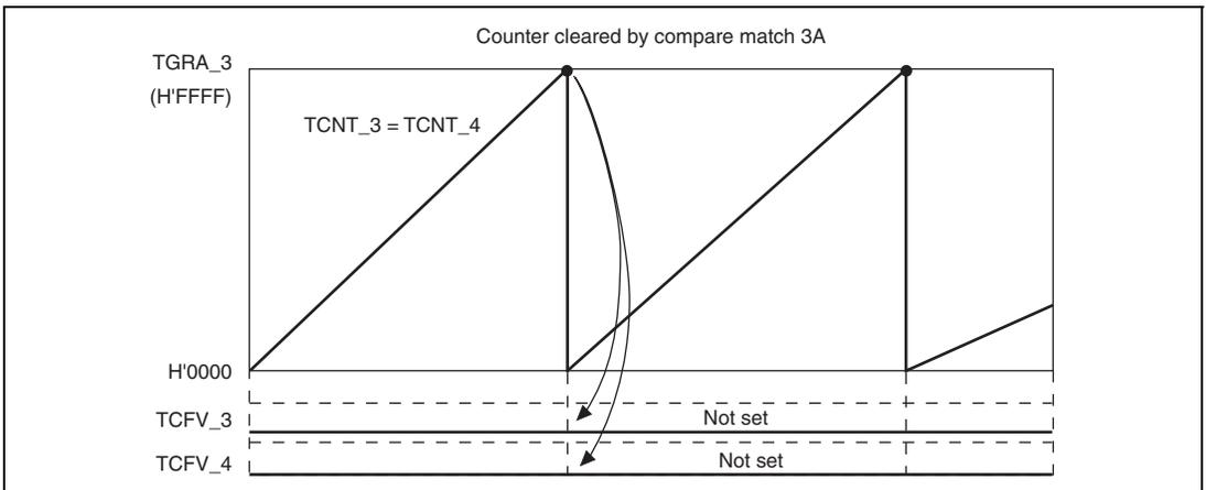
**Figure 9.121 Reset Synchronous PWM Mode Overflow Flag**
