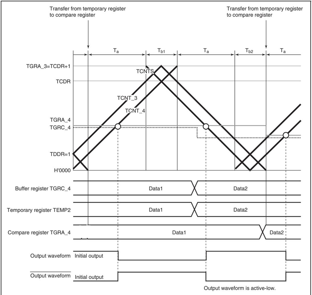
**Figure 9.41 Example of Operation without Dead Time**
