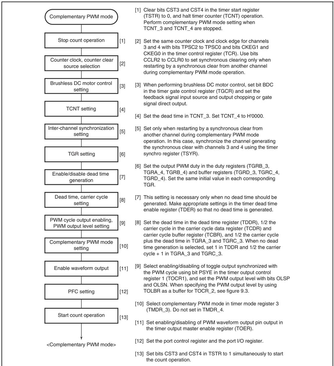
**Figure 9.38 Example of Complementary PWM Mode Setting Procedure**
