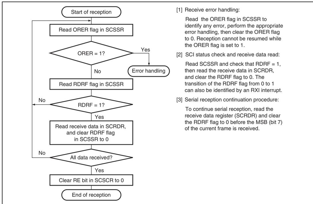
**Figure 12.12 Sample Flowchart for Receiving Serial Data (1)**
