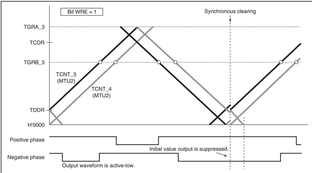
**Figure 9.61 Example of Synchronous Clearing in Interval Tb at Trough
