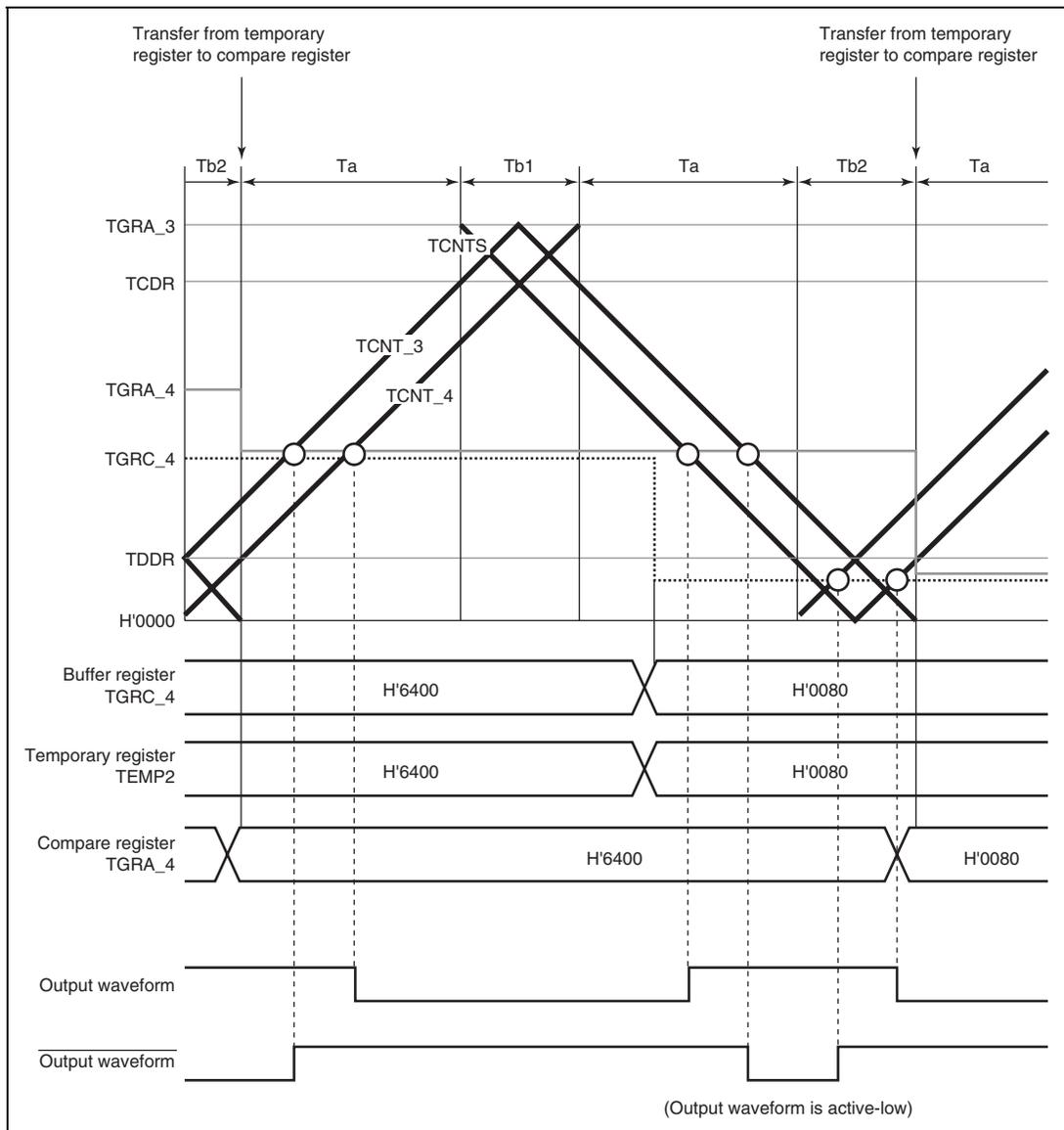
**Figure 9.40 Example of Complementary PWM Mode Operation**
