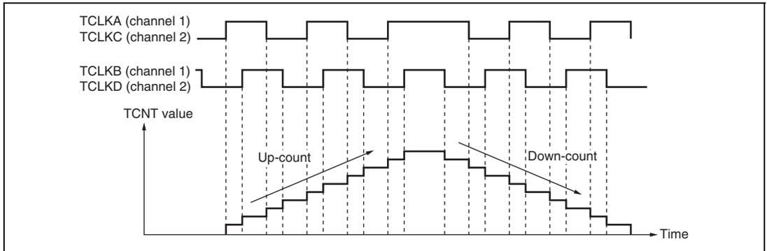
**Figure 9.30 Example of Phase Counting Mode 1 Operation**
