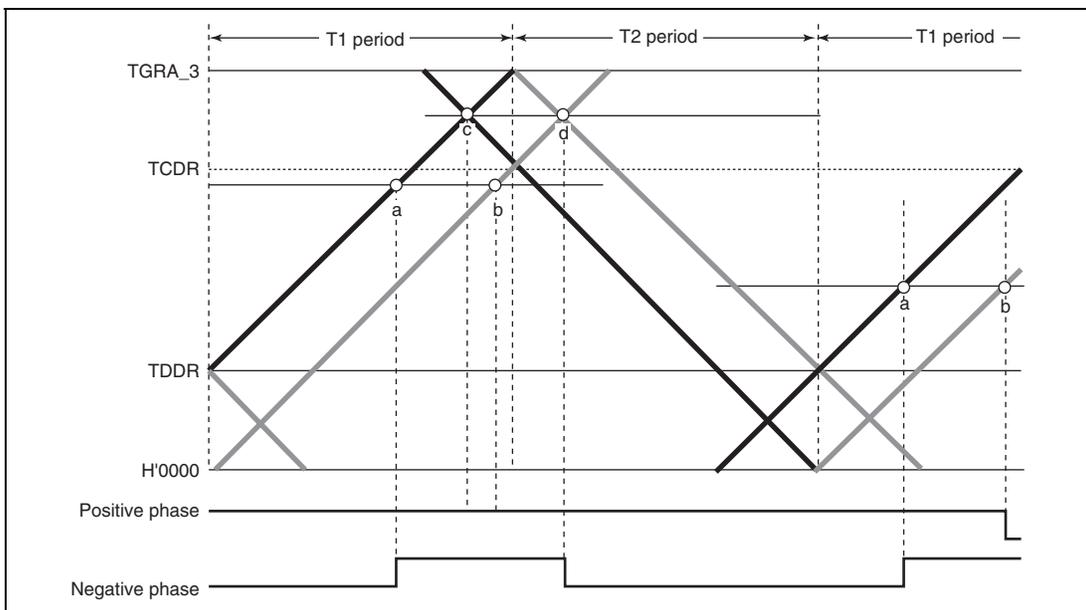
**Figure 9.47 Example of Complementary PWM Mode Waveform Output (2)**
