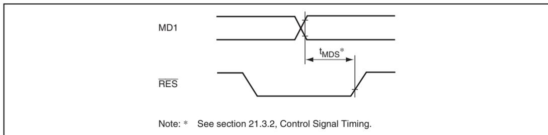
**Figure 3.5 Reset Input Timing when Changing Operating Mode**
