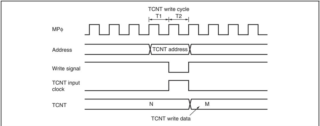
**Figure 9.109 Contention between TCNT Write and Increment Operations**
