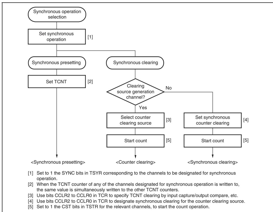
**Figure 9.12 Example of Synchronous Operation Setting Procedure**
