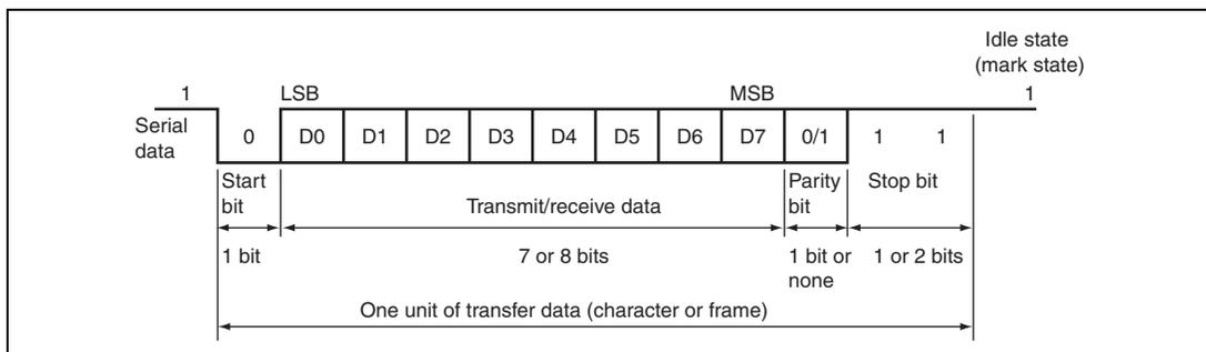
**Figure 12.2 Example of Data Format in Asynchronous Communication
