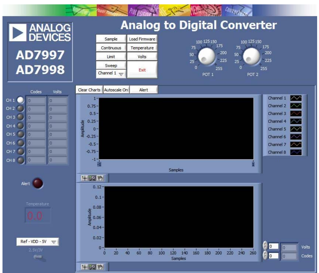
Figure 2. AD7997/AD7998 Evaluation Board Window
