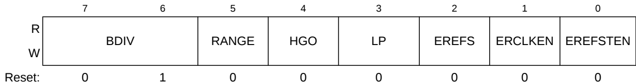
Figure 8-4. MCG Control Register 2 (MCGC2)
