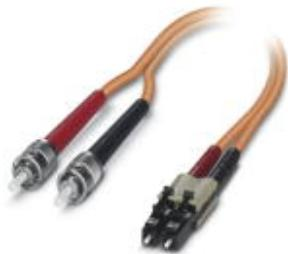
Assembled FO cable, zip cord cable, multi-mode fiberglass 50/125 µm, OM2, plug: LC/B-FOC (ST), degree of protection: IP20, for installation in cable ducts or control cabinets, length: 2 m
