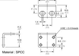
2 pieces of M2 $\times$ 4mm .157inch and 2 pieces of M2 $\times$ 8mm .315inch pan head screws are attached
