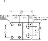
Material : SPCC 2 pieces of M2×4mm .157inch pan head screws are attached
