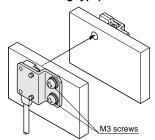
• UZB802 (SPCC) (mounting bracket for the side sensing type)
