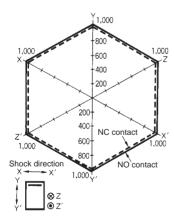
Condition: The Units were shocked at the rate of 500 m/s<sup>2</sup> (approximately 50G) three times each in the  $\pm X$ ,  $\pm Y$ , and ±Z directions with and without voltage imposed on the Units until the Units malfunctioned.
