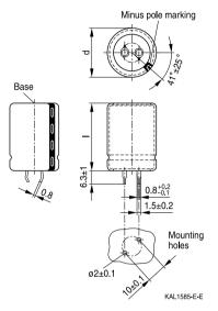
Snap-in terminals, length ( $6.3\pm1$ ) mm. Also available in a shorter version with a length of (4.5-1) mm. PET insulation is marked with label "PET" on the sleeve. Safety vent on the case wall.
