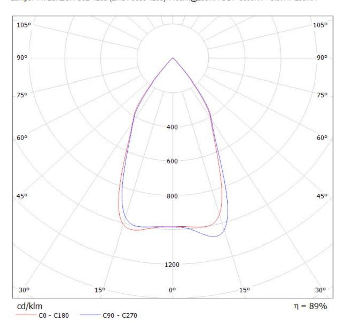
Luminaire: LEDiL Oy CN12649\_LENINA-W-DL\_(LUXEON\_CoB\_1205) Eff: 84 % Lamps: 1 x LUXEON CoB 1205 (LHC1-3080-1205) 1106lm@250mA CCT=3000K P=8.3W I=250mA
