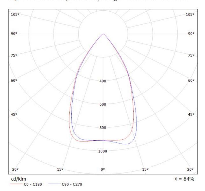
Luminaire: LEDiL Oy CN12962\_LENINA-XW\_(Luxeon\_CoB\_1205) Eff: 90 % Lamps: 1 x LUXEON CoB 1205 (LHC1-3080-1205) 1106lm@250mA CCT=3000K P=8.3W I=250mA
