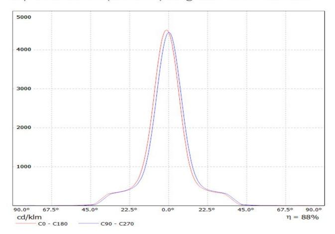
Luminaire: LEDiL Oy CN12647\_LENINA-S-DL\_(LUXEON\_CoB\_1205) Eff: 84 % Lamps: 1 x LUXEON CoB 1205 (LHC1-3080-1205) 1106lm@250mA CCT=3000K P=8.3W I=250mA
