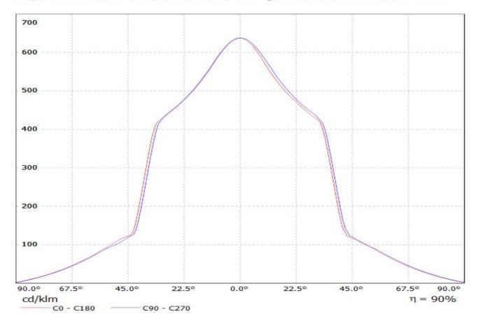
Luminaire: LEDiL Oy CN12644\_LENINA-S\_(LUXEON\_CoB\_1205) Eff: 88 % Lamps: 1 x LUXEON CoB 1205 (LHC1-3080-1205) 1106lm@250mA CCT=3000K P=8.3W I=250mA
