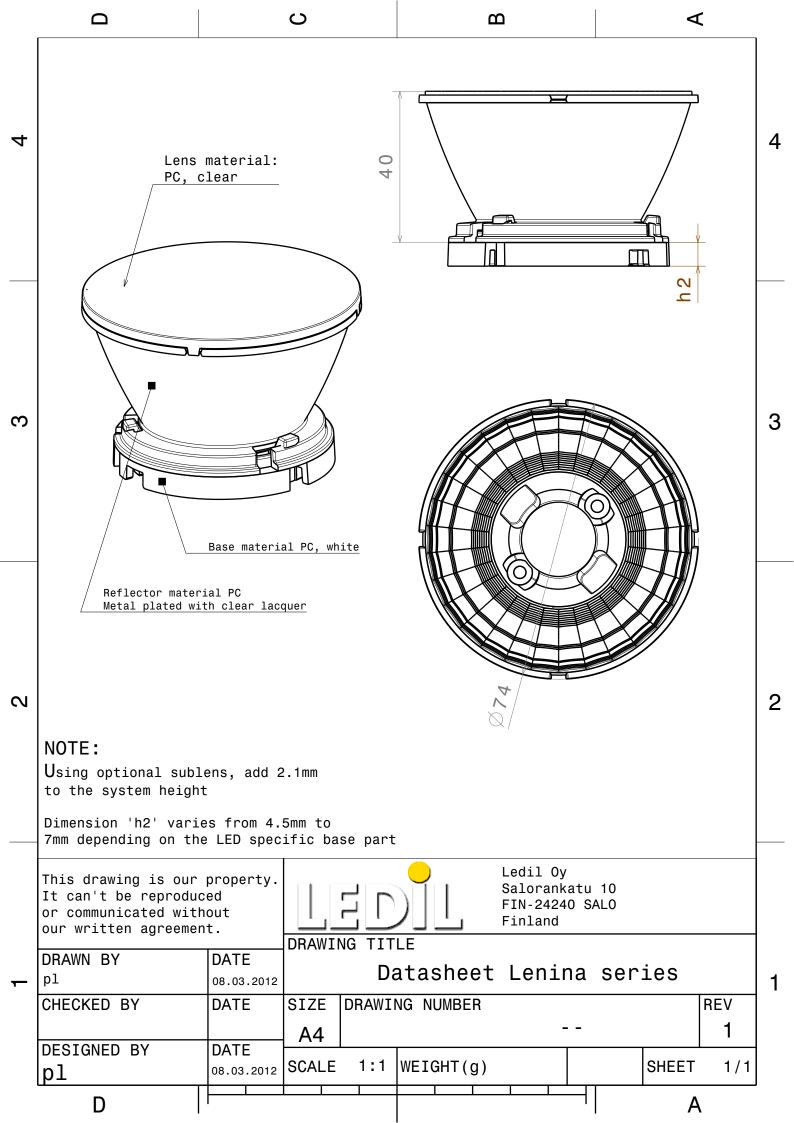
Luminaire: LEDiL Oy CN12644\_LENINA-S\_(LUXEON\_CoB\_1205) Eff: 88 % Lamps: 1 x LUXEON CoB 1205 (LHC1-3080-1205) 1106lm@250mA CCT=3000K P=8.3W I=250mA
