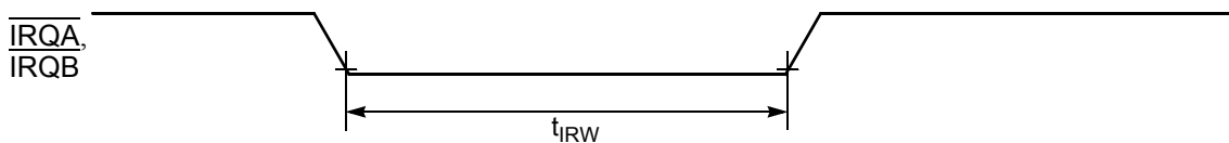
Figure 10-7 External Interrupt Timing (Negative Edge-Sensitive)
