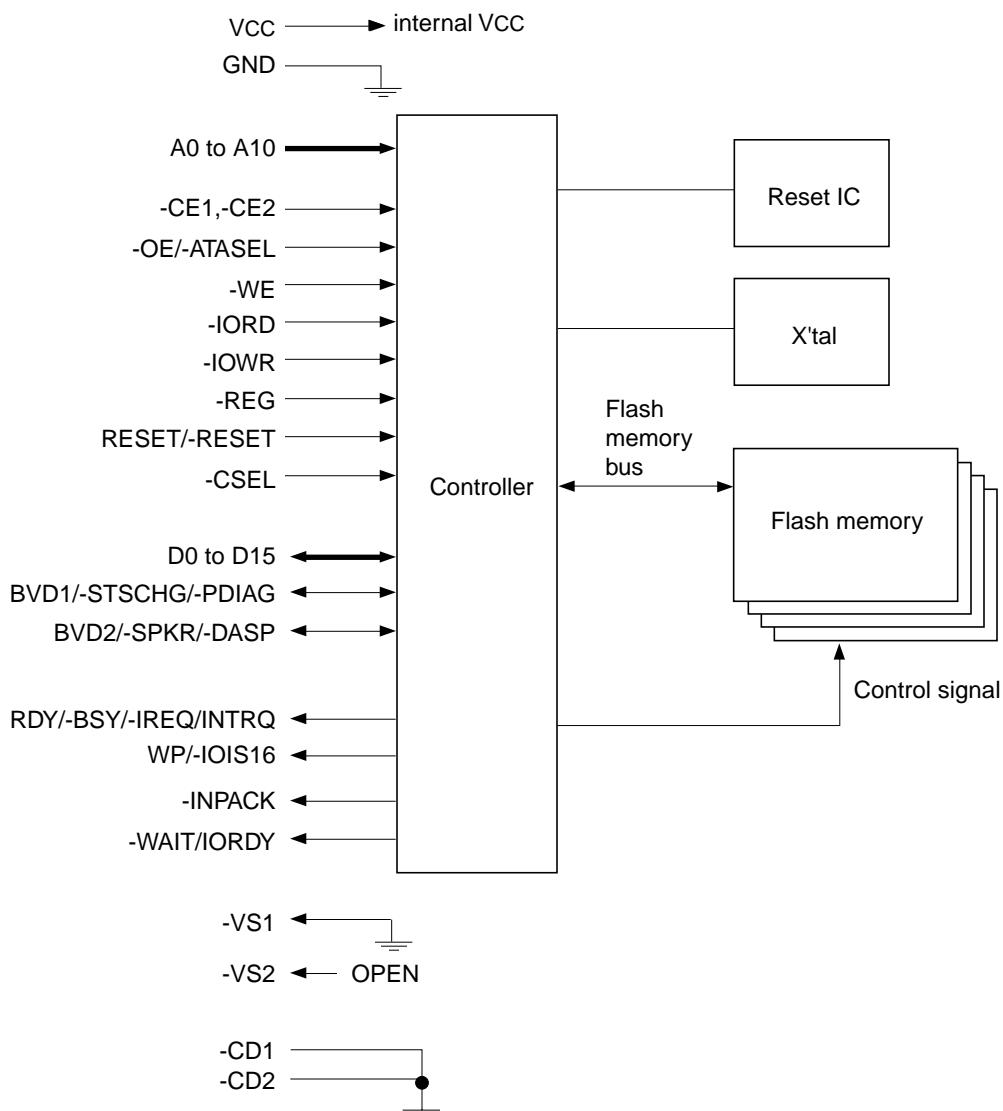
Note: -CE1, -CE2, -OE, -WE, -IORD, -IOWR, -REG, RESET, -CSEL, -PDIAG, -DASP pins are pulled up in card.
