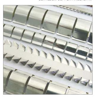
For maximum contact and shielding performance 25% compression is recommended. The standard finish is tin or bright copper, but special plating such as nickel or zinc with clear passivation can be specified to ensure galvanic compatibility. Fingerstrip can be ordered in Clean & Bright (C) or Tinned (T) as standard. Other finishes can be specified on request.
