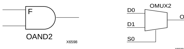
Figure 20: AND & MUX Symbols in XC4000X IOB
