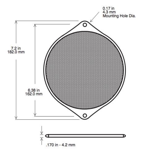
Aluminum/Stainless filters offer high levels of air passage while efficiently filtering contaminants and shielding EMI/RFI.
