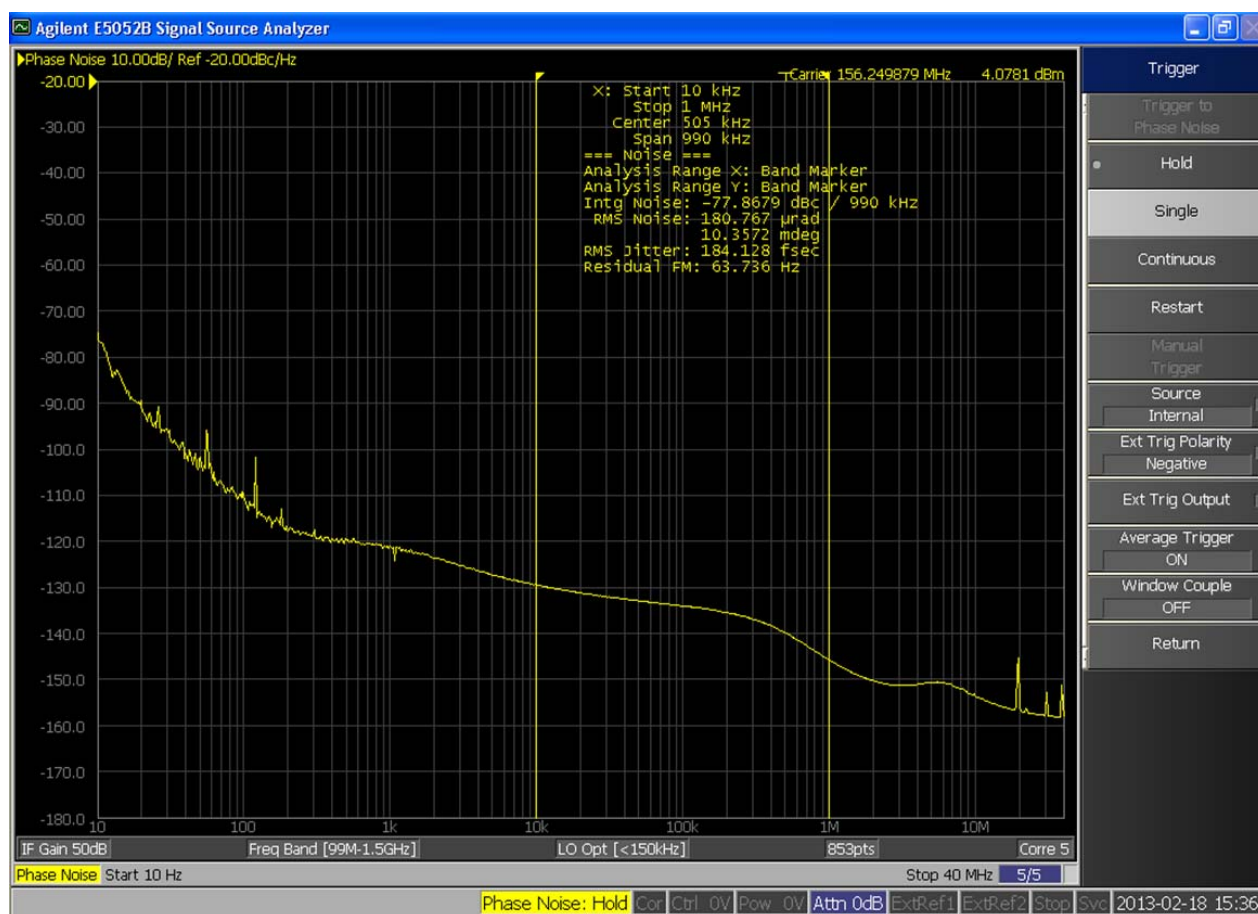
Figure 1. Si535/536 Typical Phase Noise at 156.25 MHz
