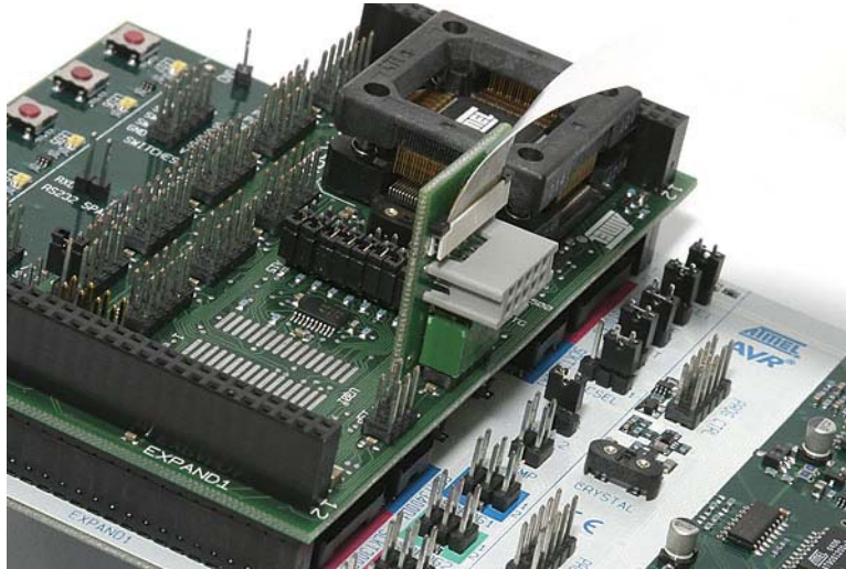
Figure 4-3: JTAG programming the AVR
