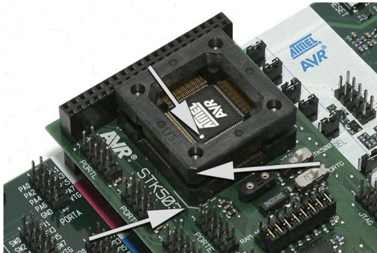
Figure 3-3: Placing the AVR in the ZIF socket.
