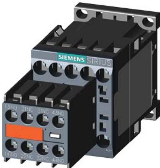
CONTACTOR, AC-3, 3KW/400V, 2NO+2NC,
