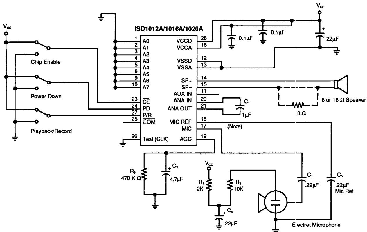
Note: If desired, this pin may be left unconnected (microphone preamplifier noise will be higher). In this case, pin 18 must not be tied to any other signal or voltage.
