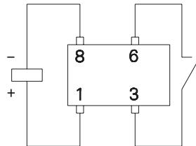
Contacts are shown in reset condition. Contact position might change during transportation and must be reset before use.
