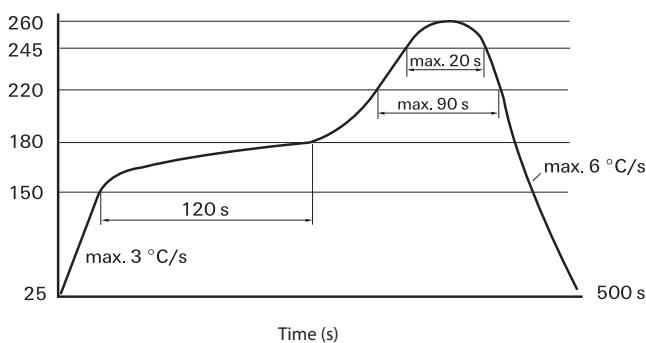
Recommended reflow soldering profile
