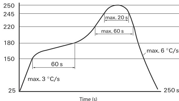
Resistance to soldering heat - Reflow profile
