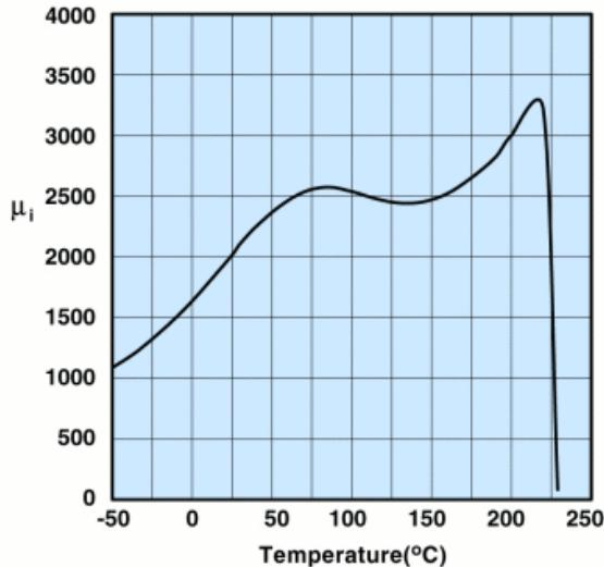
Measured on an 18/10/6mm toroid at 100kHz.
