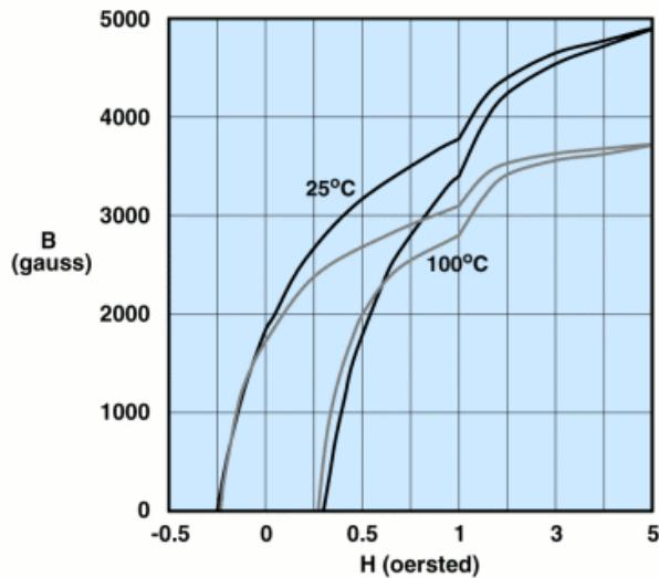
Measured on an 18/10/6mm toroid at 10kHz.
