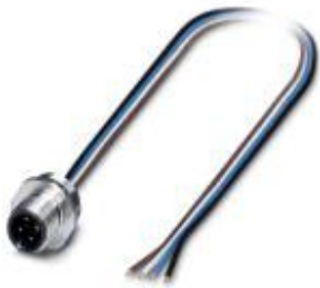
Sensor/actuator flush-type plug, 4-pos., M12, A-coded, front/screw mounting with Pg9 thread, with 0.5 m TPE litz wire, 4 x 0.34 mm², stainless steel version
