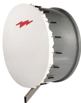
1.8 m | 6 ft High Performance Parabolic Shielded Antenna, single-polarized, 7.125–8.500 GHz, PDR84, gray antenna, standard white radome with flash, standard pack—one-piece reflector
