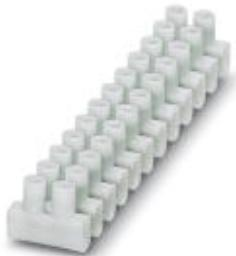
Polypropylene Europe terminal strip, white, for connecting solid conductors and stranded conductors with and without ferrules with a cross section of 0.75 to 6 mm<sup>2</sup>
