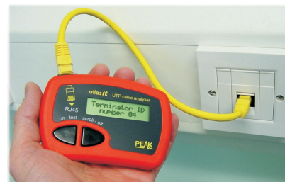
Identify multiple cable runs with the optional identified terminators
