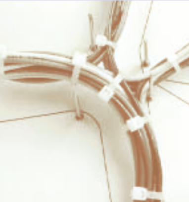
Wire and Cable Bundling (Harnessing)
