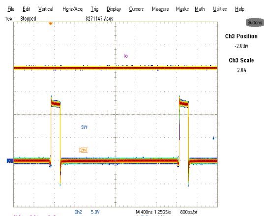
Fig. 18: Inductor node at 8A, sourcing current, Ch3:SW, Ch4:I out
