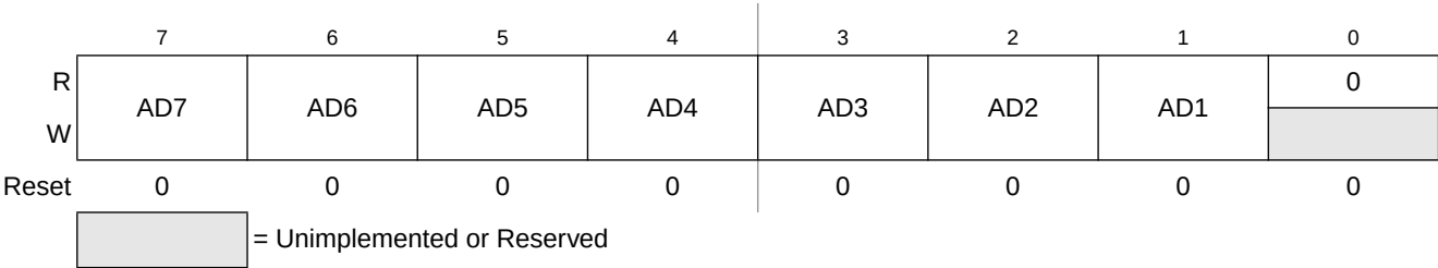
Figure 11-3. IIC Address Register (IICxA)
