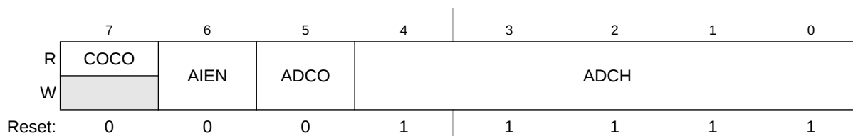
Figure 10-3. Status and Control Register (ADCSC1)
