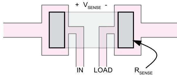
Choose a low inductance type sense resistor if preservation of bandwidth is important. The use of Kelvin connections helps by excluding the inductive voltage drop across the traces leading to the sense resistor. The inductive voltage drop may be substantial when operating at high frequencies.
