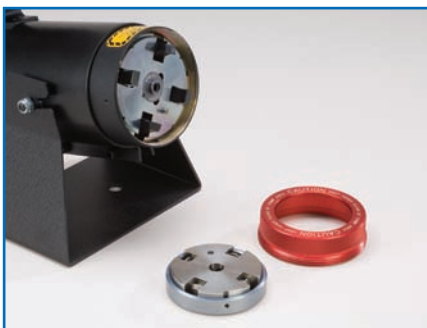
2. Pull off Indenter Die Assembly by hand.
