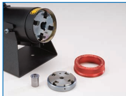
3. Pull out the Locator by hand.
