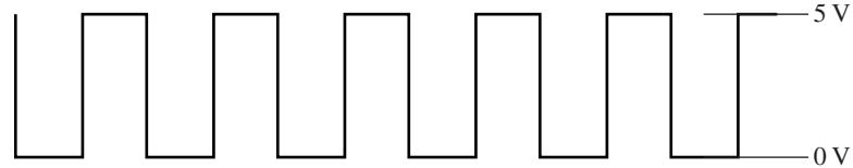
A square wave signal with a 50% duty cycle, oscillating between 0 V and 5 V. The period is approximately 16 ms.          |
