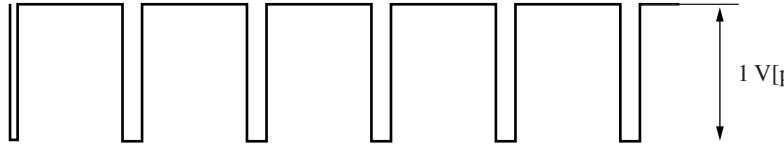
A square wave signal with a low period of 1 $\mu$ s, oscillating between 0 V and 1 V. The period is approximately 2 $\mu$ s. |
