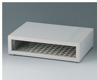
B2211007 MEDITEC D 160, without handle bar ABS (UL 94 HB) off-white RAL 9002 11.42"x7.87"x2.91" IP 40
