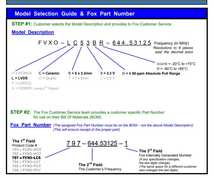
This example, FVXO-LC53BR-644.53125 = Voltage Controlled, LVDS Output, Ceramic, 5 x 3.2mm Package, 3.3V, ±50 PPM Absolute Pull Range, -40 to +85°C Temperature Range, at 644.53125 MHz
