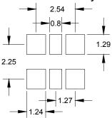
Note: XPRESSO LVDS VCXOs are designed to fit on Industry standard, 6 pad, layouts.
