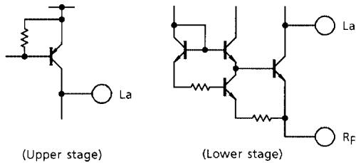
This circuit uses the power transistor's base current to regulate the circuit's output current.
