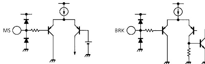
When  $V_C > V_{ref}$ , one of three modes (Reverse Rotation, Reversing Brake or Short Brake mode) can be selected by setting the MS and BRK pins appropriately.
