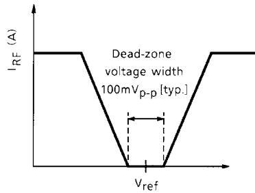
$$gm = \frac{\Delta I_{RF}}{\Delta V_C} = 1.0[A/V] \text{ (typ.)} \text{ (at } R_F = 0.3\Omega \text{)}$$
