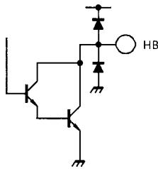
The hall element bias current is turned off when the driver IC is in standby state.
