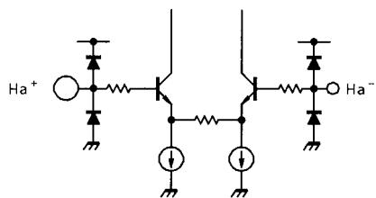
The common mode input voltage range for VCMRH is 1.5 to 4.0 V.
