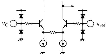
The Common mode input voltage ranges for both  $V_C$  and  $V_{ref}$  are 1.0 to 4.0 V.
