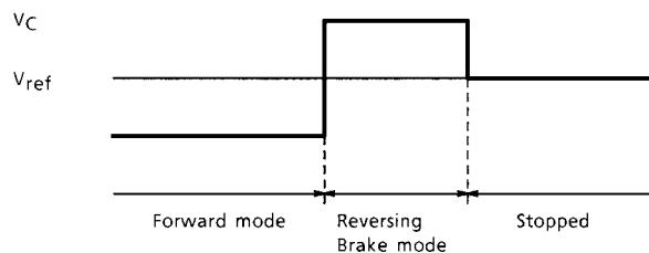
Note: For an explanation of the Reversing Brake mode stopping sequence, refer to the explanation of the reverse rotation detection circuit.
