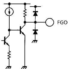
This circuit uses a hall element signal which is output to FGO after a Schmitt stage.
