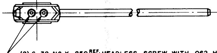
(2) 6-32 NC X .250<sup>REF</sup> HEADLESS SCREW WITH .062 HEX. SOCKET.
