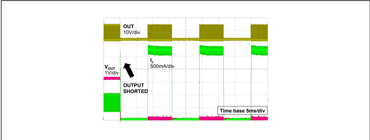
Figure 32. Short-circuit behavior
