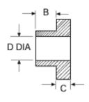
Note: A single gate extension, not to exceed 0.64mm (0.025") in length, is allowable on the outside of all shoulder washers.
