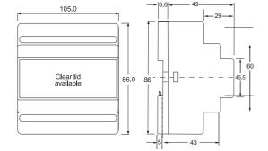
Module enclosure for M36 DIN-rail.
