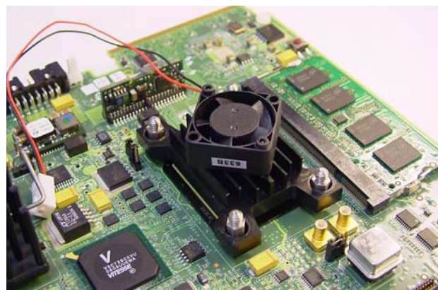
Figure 7-3. Remove Allen Screws
