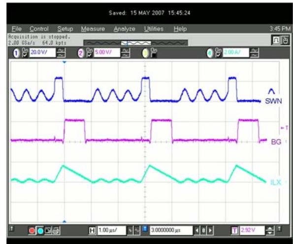
Figure 23. Switcher Operation – DCM Mode
