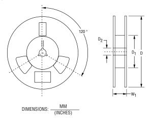
Devices are packed in accordance with EIA standard RS-481-A.
