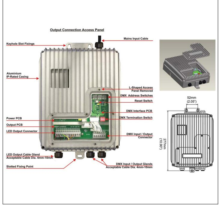
Note: The min/max wires that the quick connect terminals can accept are wire gauge:  $Min = 0.08mm^2$  (0.32mm dia.) Max = 2.5 $mm^2$  (1.8mm dia.)
