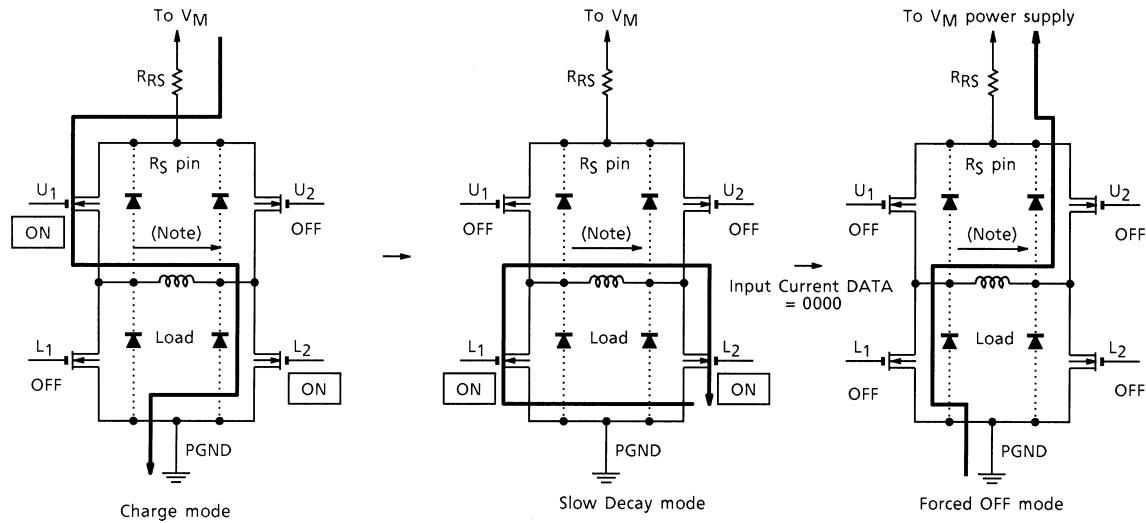
As shown in the figure at right, an output transistor has parasitic diodes.
