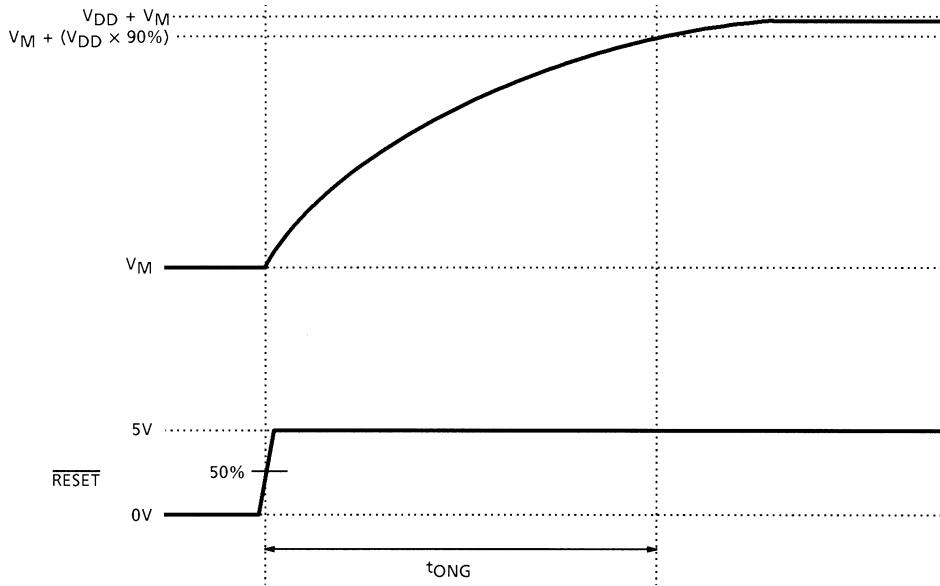
$t_{TONG}$ : Time taken for capacitor Ccp2 (charging capacitor) to fill up Ccp1 (capacitor used to save charge) to  $V_M + VDD$  after a reset is released.
