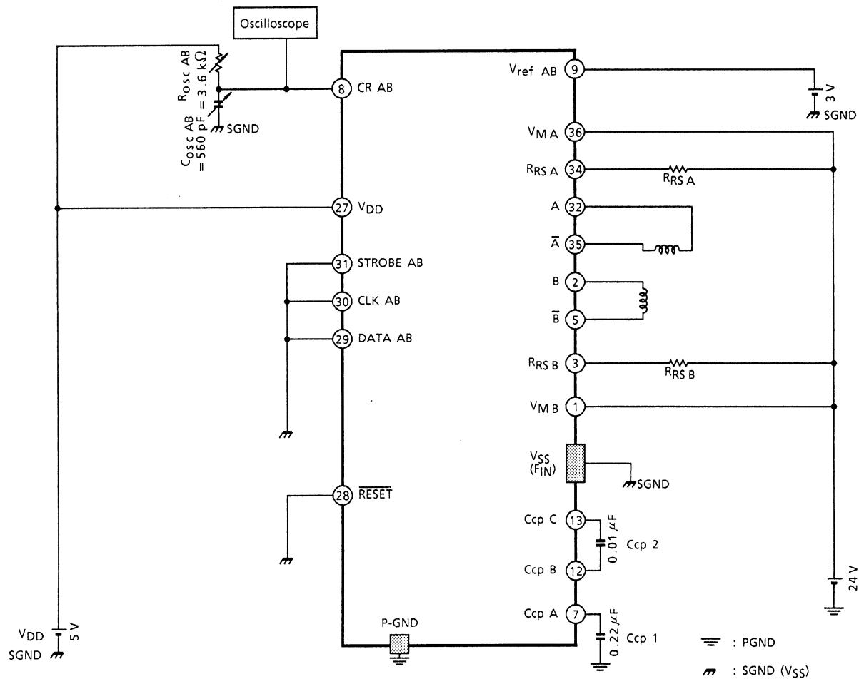
Change the  $R_{osc}$  and  $C_{osc}$  values and measure the frequency on the CR pin using the oscilloscope.
