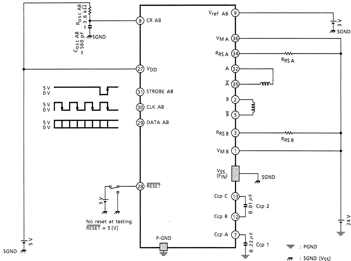
tBRANK is the dead time band for avoiding malfunction caused by noise. Apply sufficient differential voltage (when  $V_{ref} = 3 V$ , 0.6 V or higher) to  $V_M$ -RS and apply duty. When the pulse width reaches a certain value, triggering feedback and changing the output. Check the value.
