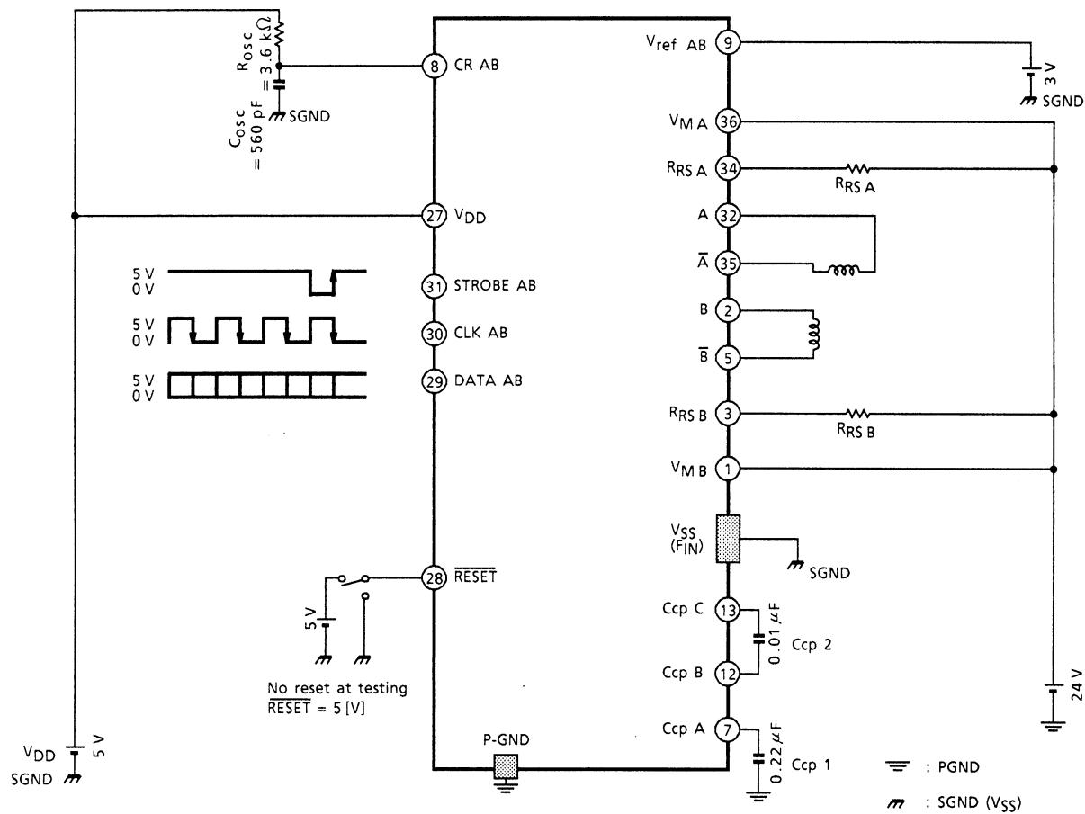
Fix the output current value in Mixed Decay mode and turn the output on. Measure the time until the output switches from the CR pin waveform and the output voltage waveform.
