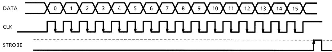
Note: Data input to the DATA pin are 16-bit serial data.
