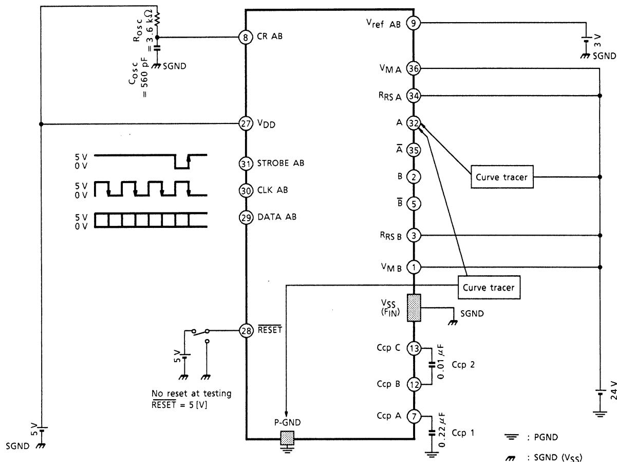
$T_jTSD$ : Increase the ambient temperature. Measure the temperature when output stops.
