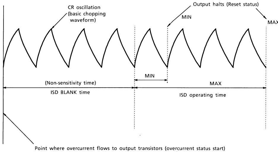
A non-sensitivity time is set for the overcurrent protector circuit to avoid misdetection of overcurrent due to spike current at irr or switching.
