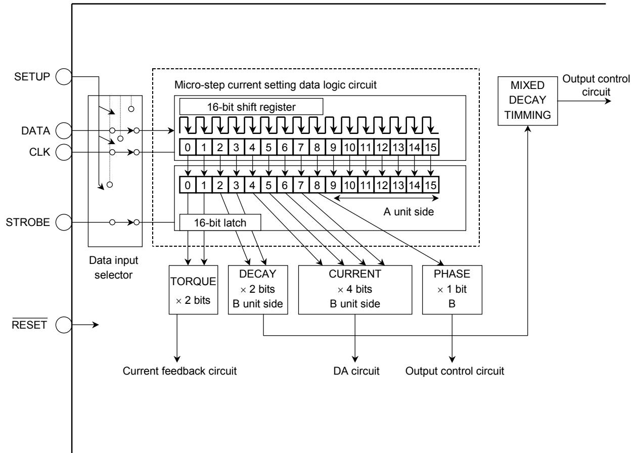
Note: The RESET and SETUP pins are pulled down in the IC by 10-k $\Omega$  resistor.
