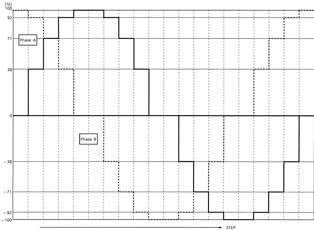
5 micro-step from 0 to 90° drive is possible by combining Current DATA (AB & CD) and phase data.
