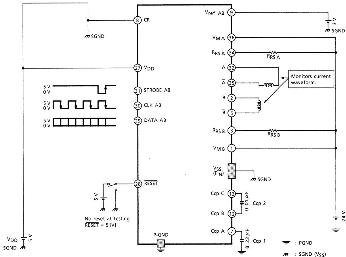
With L load, perform chopping in Mixed Decay mode. Monitor the output current waveform and measure the various output currents at constant current operation.
