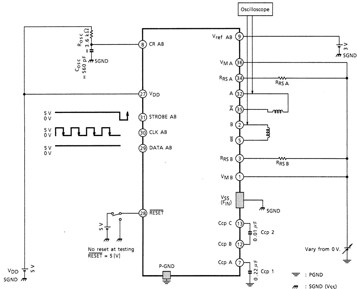
With the CLK signal and DATA (all High) input, increase the VM voltage from 0.
