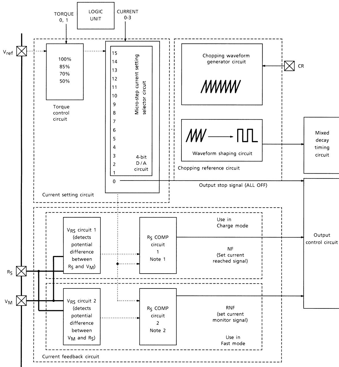
Note 1: RS COMP 1: Compares the set current with the output current and outputs a signal when the output current reaches the set current.
