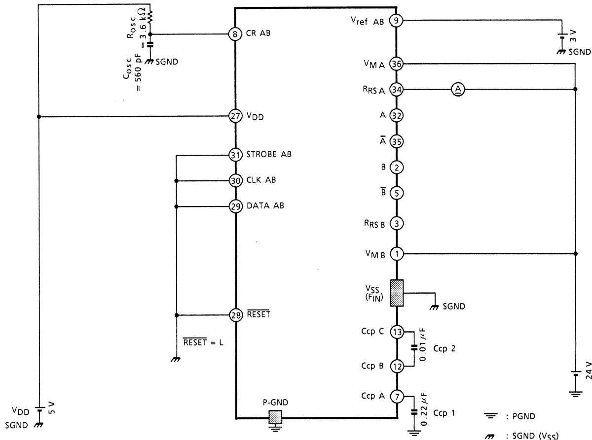
With L input to RESET, connect VM and RRS to the power supply, and measure the current input to the RS pin. (Either drop all the input pins to GND level or input all Low data to the DATA pin, then perform measurement. At that time, leave all other output pins open.)
