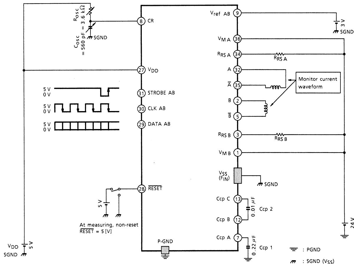
Perform chopping in Mixed Decay mode with load L. Monitor the output current waveform and measure the output current at constant current operation. At this time, vary the 4-bit data for current setting and measure the current values. Using the set output current as 100%, calculate the output current ratio.
