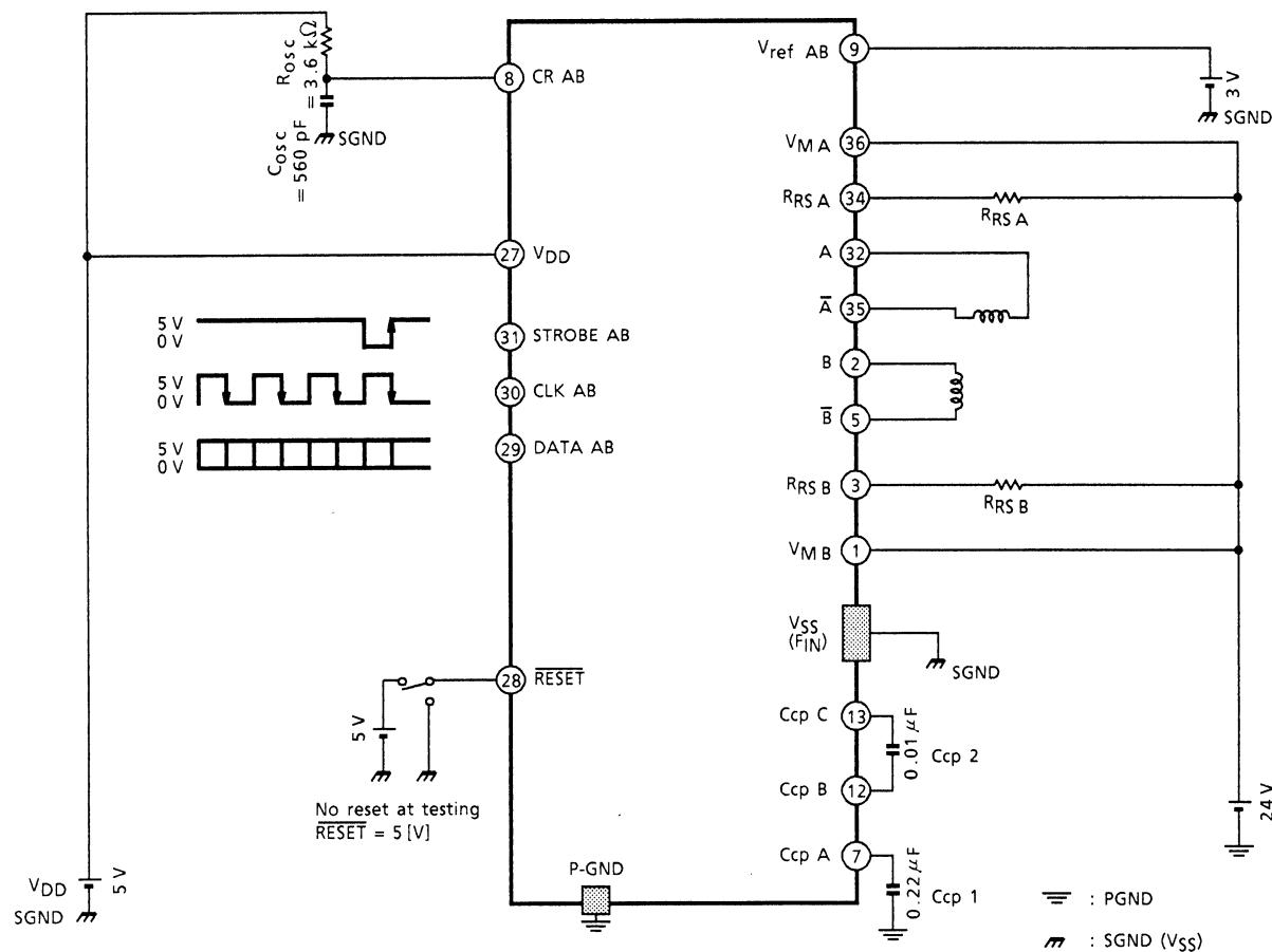
Input any data at  $f_{CLK}$  (max), perform chopping, and monitor the output waveform. For the measuring points, see the timing chart below.
