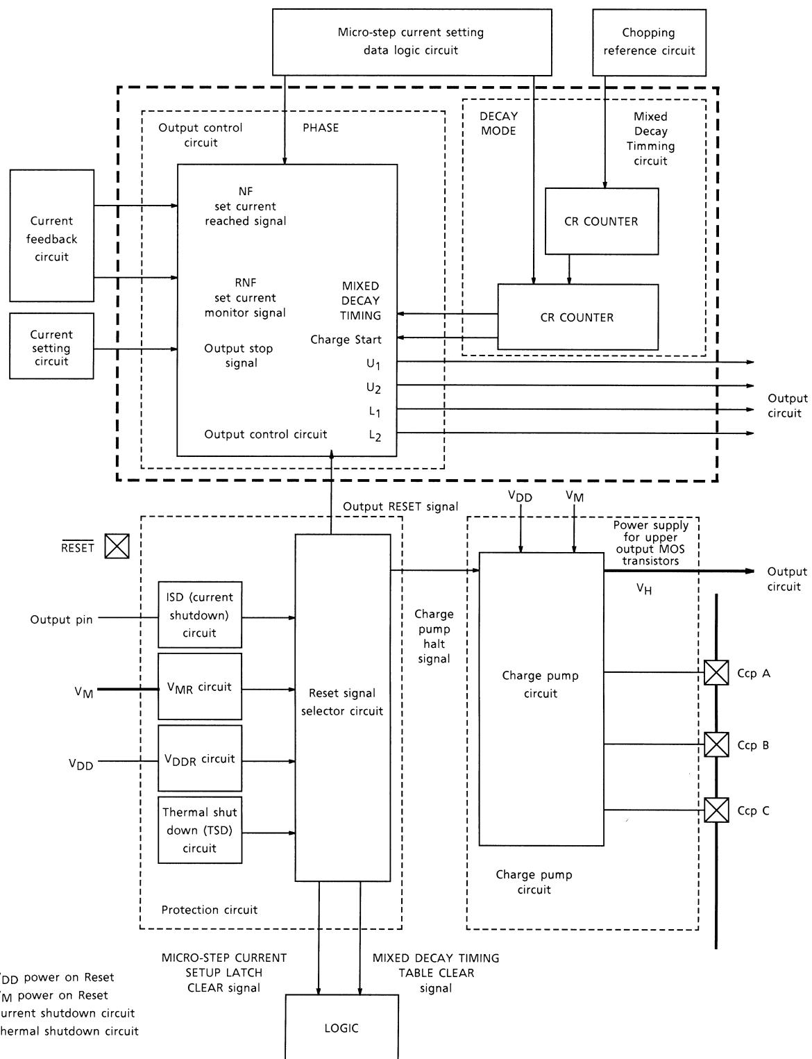
Note: The RESET pins is pulled down in the IC by 10-k $\Omega$  resistor.
