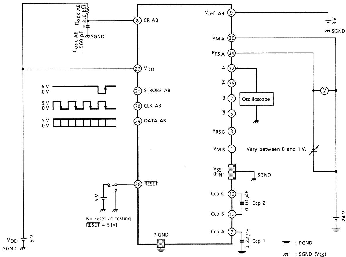
$V_{RS}$  (H to L): Input torque data = 100% (HH) and vary the voltage between  $V_M$  and  $R_S$  pins.
