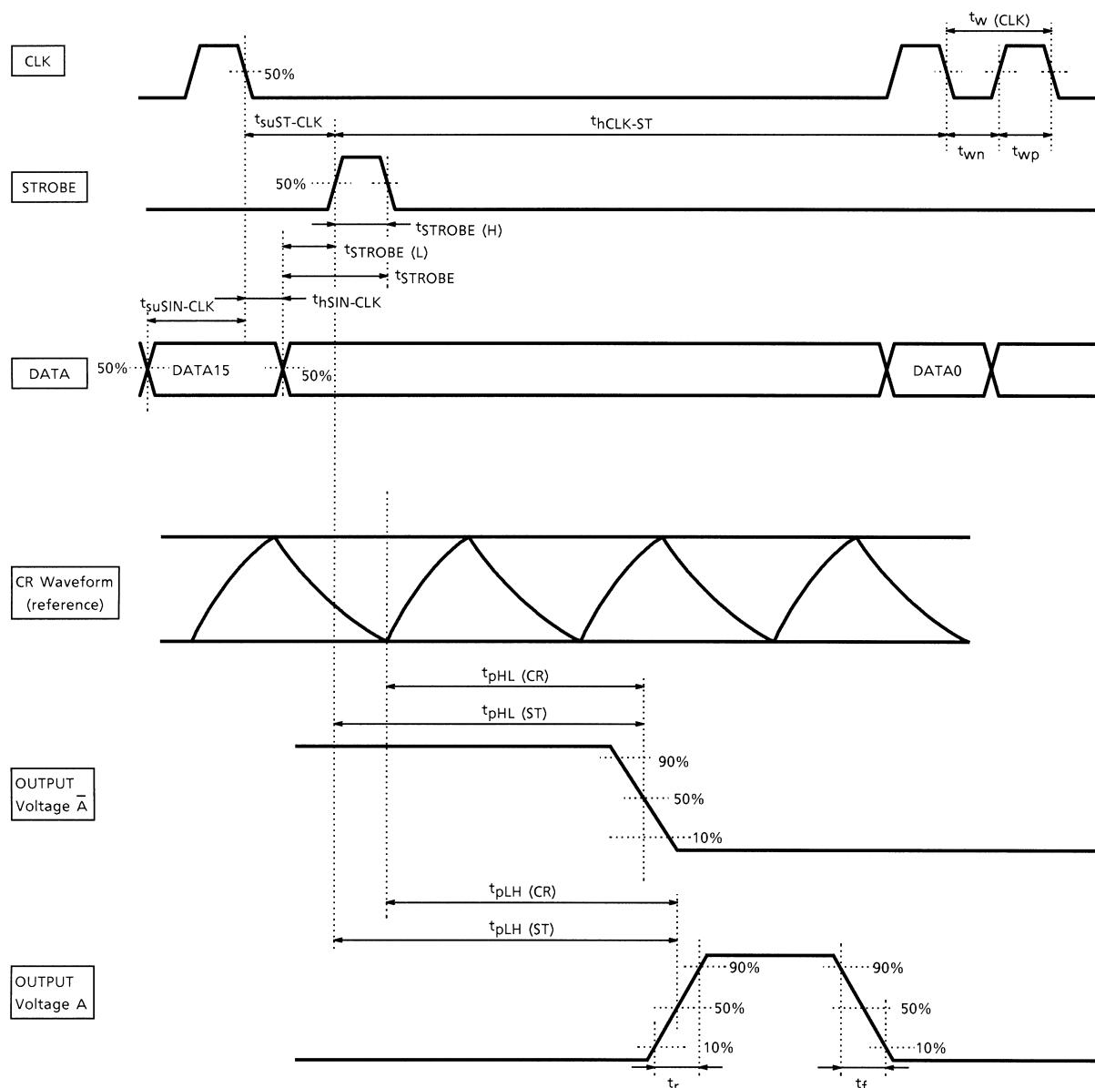
**Test Waveforms (Timing waveforms and names)**
