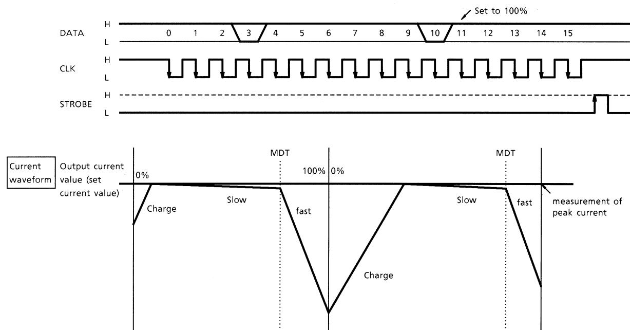
8.  $I_{RS}$  (when measuring phase A) (A/B unit only. C/D unit conforms to A/B unit)
