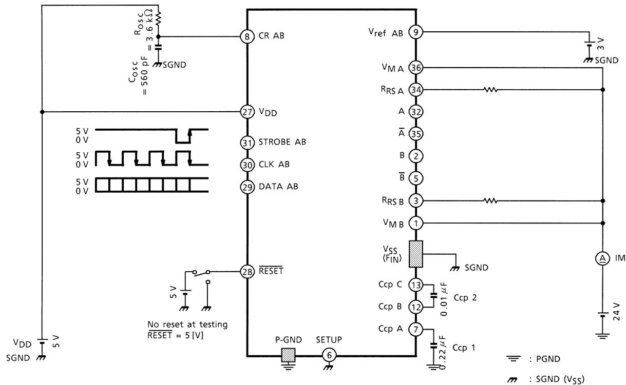
This is the IM current when all of the circuits, including the output transistors, in the IC are operating. The IM current includes the current dissipation in the charge pump circuit, output gate loss, and output predriver.
