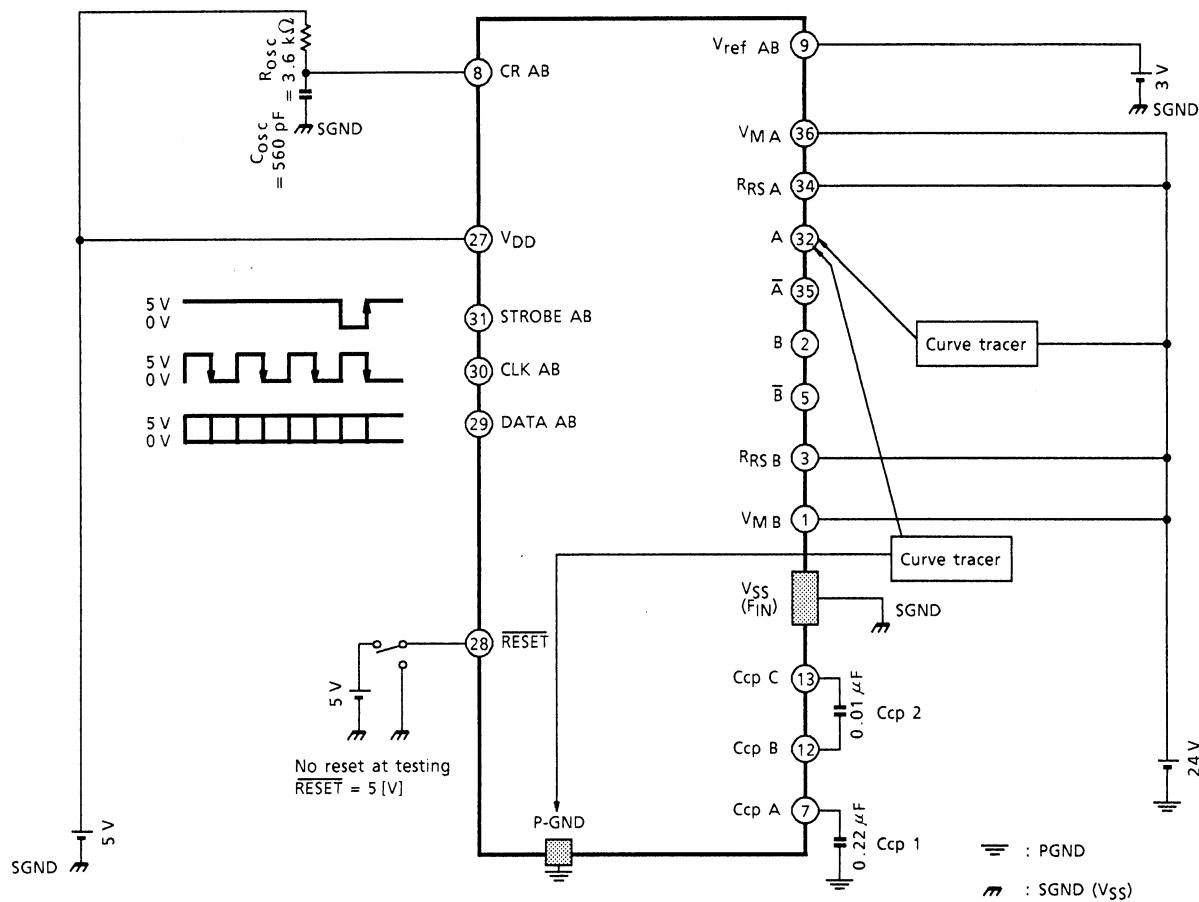
Input the current setting data (HHHH signal) to the DATA pin and measure the voltage between VM and OUT when  $I_{out} = 1000$  mA or the voltage between OUT and GND. Then, change the phase and repeat measurement. At that time, leave the output pins which are not measured open.
