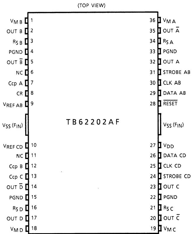
Note: [Important] If this IC is inserted reverse, voltages exceeding the voltages of standard may be applied to some pins, causing damage.
