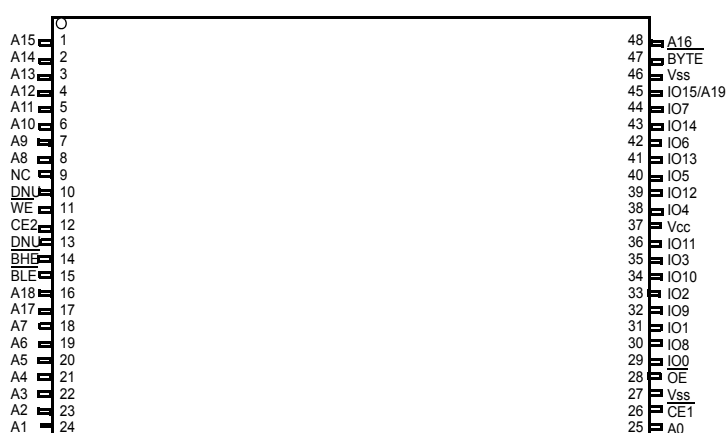
48-Pin TSOP I (512K x 16 / 1M x 8) Top View
