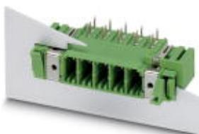
Feed-through header, nominal current: 41 A, rated voltage (III/2): 630 V, nominal cross section: 6 mm<sup>2</sup>, number of positions: 12, pitch: 7.62 mm, color: green, contact surface: Tin, mounting: Wave soldering, pin layout: Linear pinning, solder pin [P]: 4.26 mm
