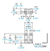
Material: Cold rolled carbon steel (SPCC)
